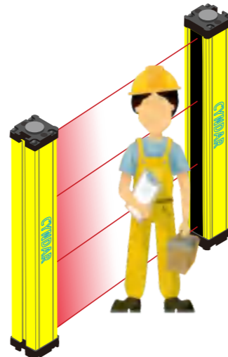
手臂或身体保护 间距30/40/80mm Arm or body protection spacing
