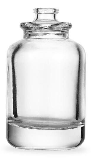
Brimful Capacity **58±2 ml** Net Weight **140±5 g** Dimensions **Dia.46.97 x H83.63 mm** Neck Finish **FEA15**
