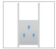
3. Attach the right aluminium rod to the coop. Push up the door by hand to ensure the door slides smoothly.
