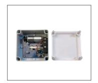
4. Open the front panel of the controller and take out the battery holder, install 4\*AA batteries in the battery holder and plug it back in.
