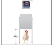
6. The door will self-check once. It will fully close and then open 30cm. The height can be adjusted by Menu button. Finally screwing the front panel to controller box.
