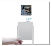
5. Attach the controller to the coop. Tie a knot on string, push the door up by hand and attach it to the string (make sure the string is vertical).
