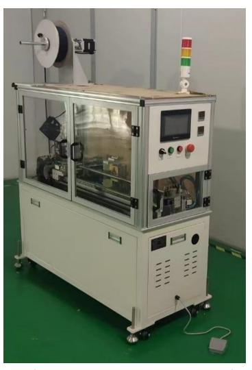
the feeding rack is on the top of machine to save the sapce and shipping cost
