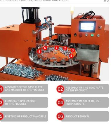
This machine is mainly used for bracket riveting of casters
