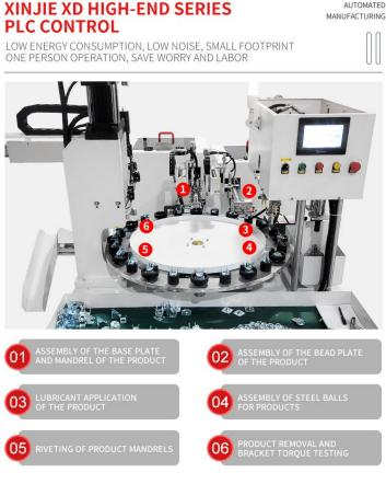
This machine is mainly used for bracket riveting of casters
