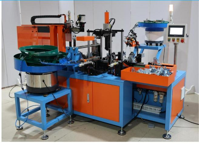
This machine is mainly for installing the brake pads of the casters
