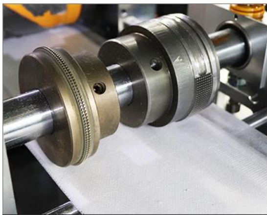
MASK UPPER EDGE PRINTING + NOSE BRIDGE WELDING
