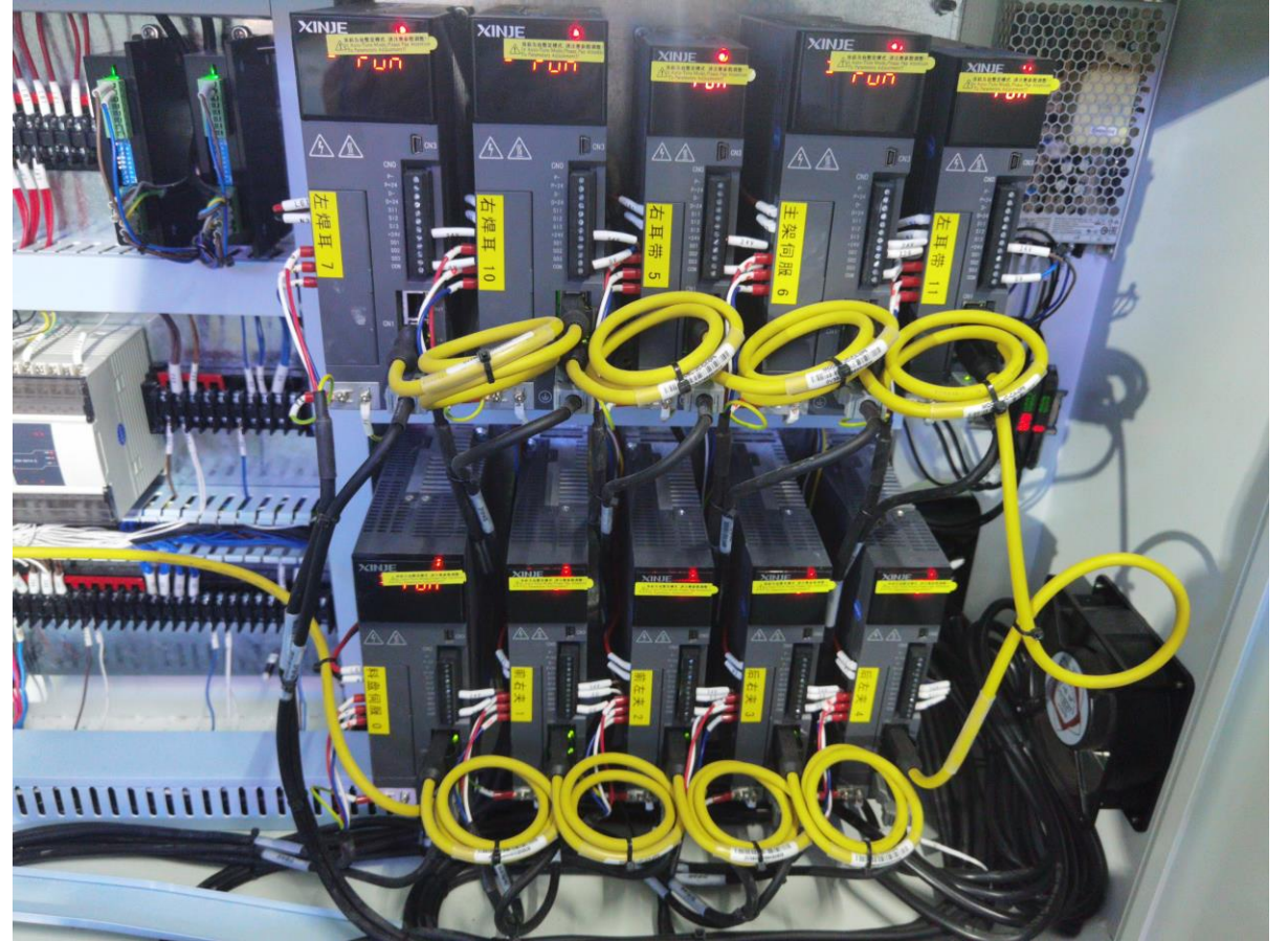
The electric box adopts bus control, with fast response speed, 5 servo motors for the film machine, and 10 servo motors for the ear band welding machine
