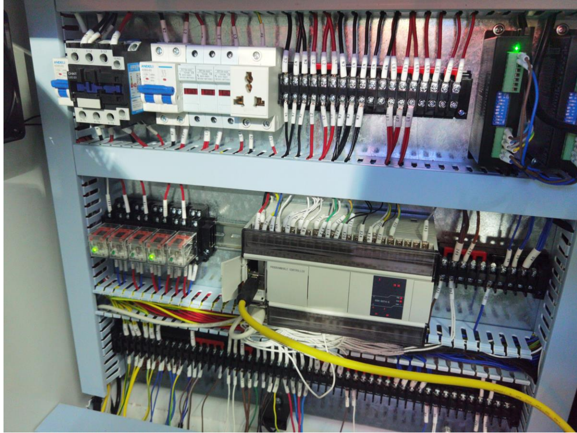
The electric box adopts bus control, with fast response speed, 5 servo motors for the film machine, and 10 servo motors for the ear band welding machine
