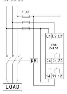
Relay contact position shown in 'Power off' condition
