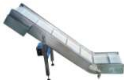
TAKE-AWAY CONVEYOR 成品输送机
