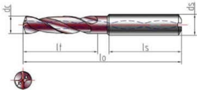
Use characteristics: used for processing common materials such as structural steel, alloy steel, stainless steel, etc.; strong centering ability, can obtain stable dimensional accuracy and good surface quality; suitable for occasions with excellent rigidity
