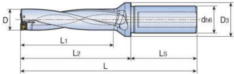
◎drilling depth: 4xD(diameter)
