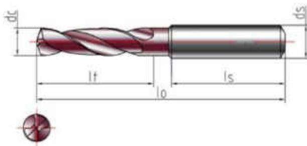
Use characteristics: used for processing common materials such as structural steel, alloy steel, stainless steel, etc.; strong centering ability, can obtain stable dimensional accuracy and good surface quality; suitable for occasions with excellent rigidity
