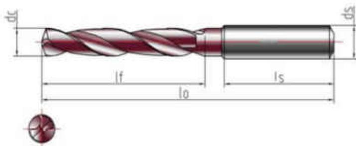
Use characteristics: used for processing common materials such as structural steel, alloy steel, stainless steel, etc.; strong centering ability, can obtain stable dimensional accuracy and good surface quality; suitable for occasions with excellent rigidity
