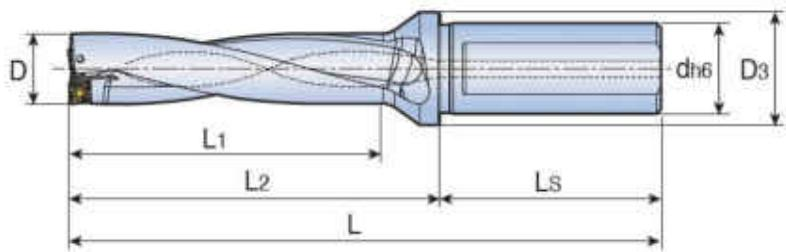
◎drilling depth: 4xD(diameter)
