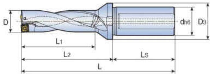
◎drilling depth: 3xD (diameter)
