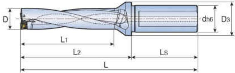
◎drilling depth: 4xD(diameter)
