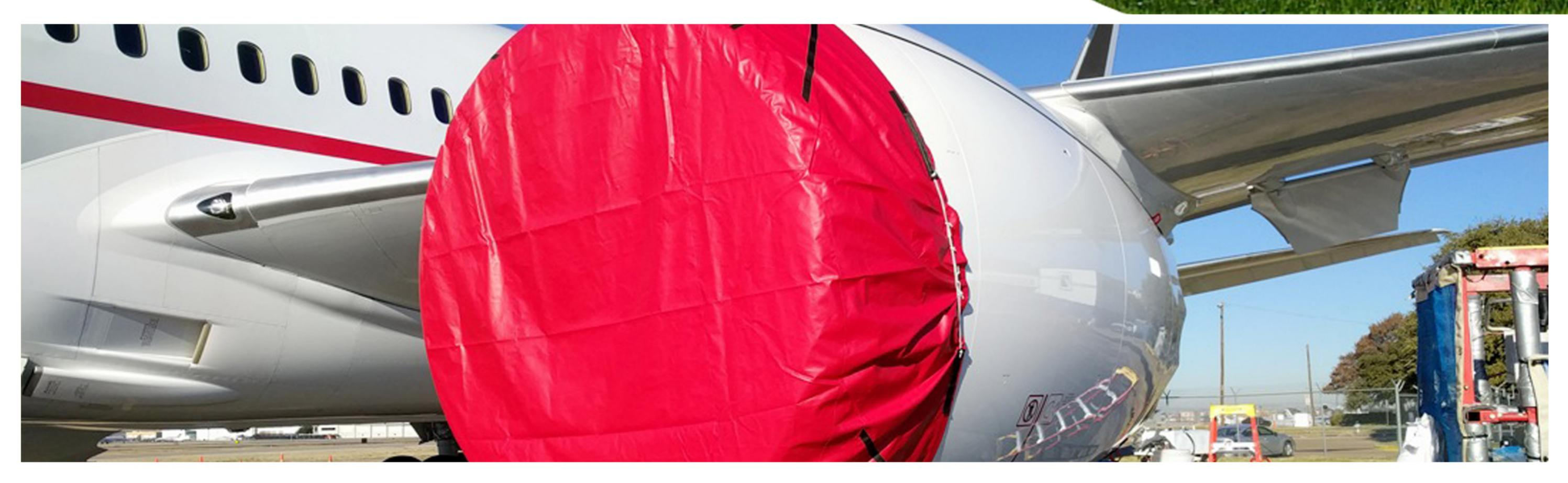
A polypropylene based fabric coated with a special polyolefin coating Container Tarpaulin makes it recyclable and weight reduction of 40% compared to PVC. High intensity, good elasticity, mildew proof, fire resistant and UV protected. Works under cold temperature, will not crack like PVC tarps. Could be hot welded.
