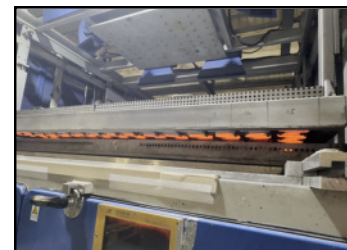
Heating to Soften
