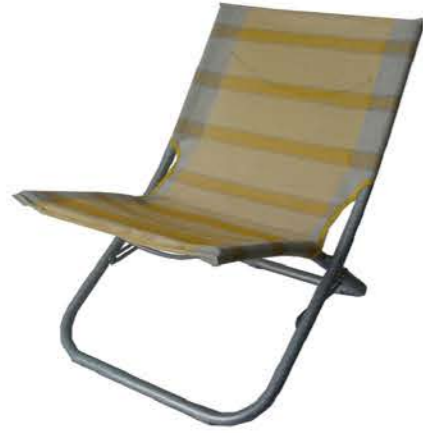
Fe YTLC018B Size: 47x64x32/58cm steel tube dia.22x0.9mm powder coated 1x1 textilene Packing 83x23x49cm 6pcs
