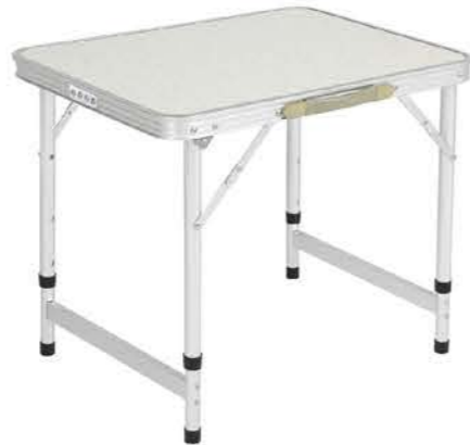
Ai ↔ YTFT110 Size: 40x45x65cm aluminum tube dia.25/23x0.8mm, oxidation 5mm MDF table top with 3.2cm width aluminum surround Packing 61.5x6.5x47.5cm 1pcs
