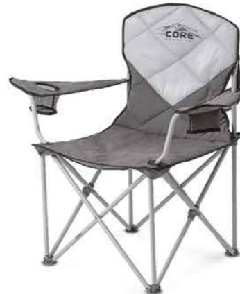
Fe ↔ ↔ YTBC145 Size: 62x62x50/90cm steel tube dia.22mm powder coated, double 600D polyester with PVC coated, 1cm thickness foam filling inside, with 1 mesh cupholder and 1 fabric cupholder, Packing 101x38x38cm 4pcs
