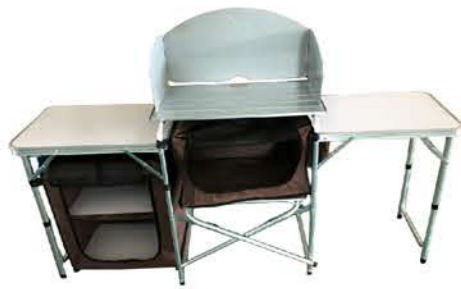
Ai ↔ YTCC058 Size: 175x46x40/70cm aluminum panel top 55x10mm, dia.19x0.8mm oxidation; 5mm MDF with 3.2cm width aluminum surround Packing 80x12x57cm 1pcs
