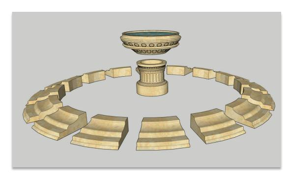
Pre-assembled the stone according to number of production drawing. Every stone piece connect with cement, and sealed the gaps with stone glue.
