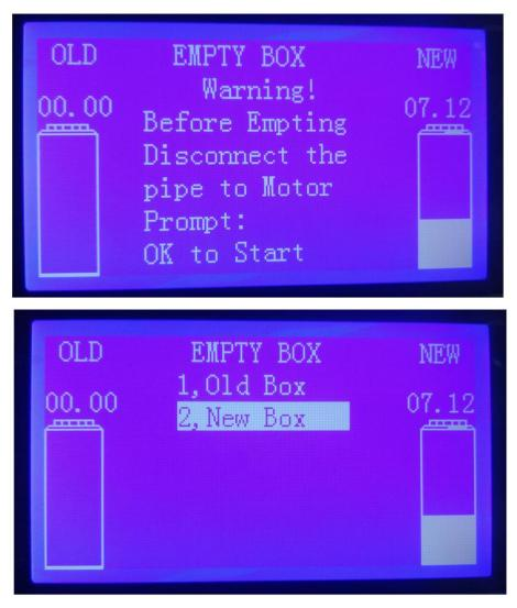
3) Use the " $\blacktriangle$ " and " $\blacktriangledown$ " buttons to select emptying the used oil tank or emptying the new oil tank. Press the "OK" button to run. Please prepare containers for keeping used oil before running.
