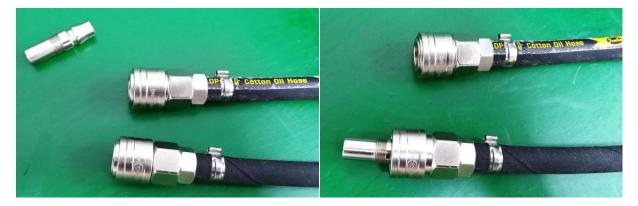
**2** Be sure to insert a small connector (arbitrary shape) on any of the two quick connectors, and only under this circumstance, the quick connector can be opened and the used oil and new oil can be discharged. Otherwise, <u>THE OIL TUBE WILL</u> <u>BURST</u>. Please note.
