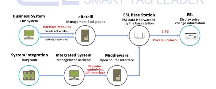
System Structure Diagram
