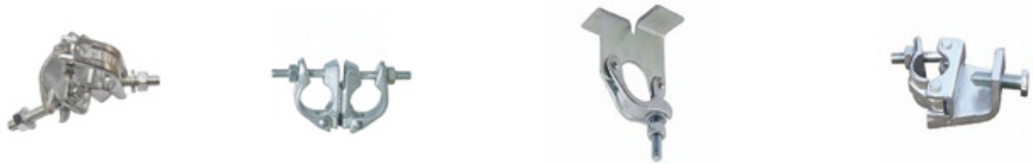
BS DF Double Coupler 48.3 mm/ 1 kg BS DF Swivel Coupler 48.3 mm/ 1.1 kg BS DF BRC(board retaining coupler) 48.3 mm/ 0.63 kg BS DF Girder Coupler 48.3 mm/ 1.5 kg
