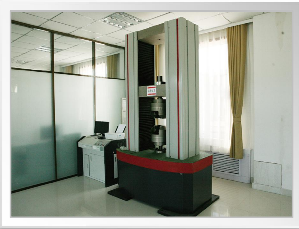
Electronic universal testing machine
