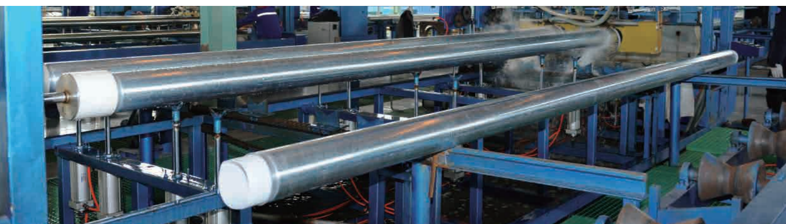
Steel Pipe of Lining Plastic Production Line
