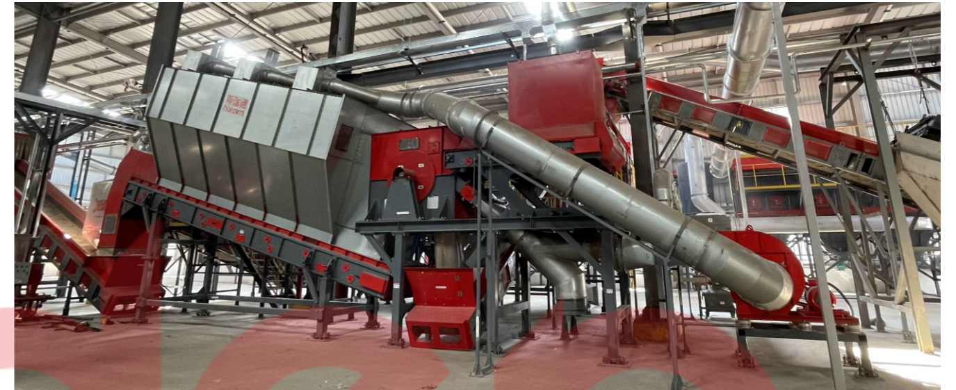
Processing materials: Industrial Waste Site: Zhangping, Fujian Province Date: Apr. 2023 Model: SFX1200 (20t/h, 40-300mm) Application: Removing impurities from RDF fuel
