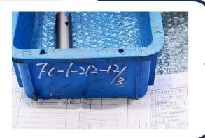
To start secondary inspection of tolerance holes and surface appearance inspection after surface treatment. If there is no other issues, put the drawings and products together into the box with labelled part number, and then transfer the box and test report to package room.
