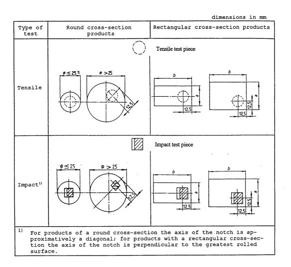
Figure 1:Position of test pieces (longitudinal test pieces)
