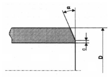
Figure 1 — Tube end bevel
