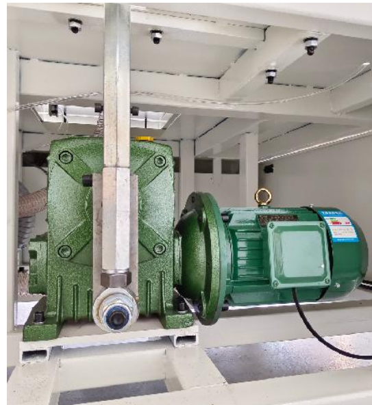
Main beam lifting gear motor
