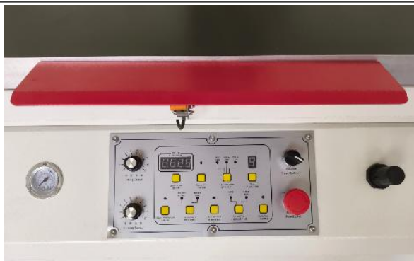
Control panel and emergency stop switch
