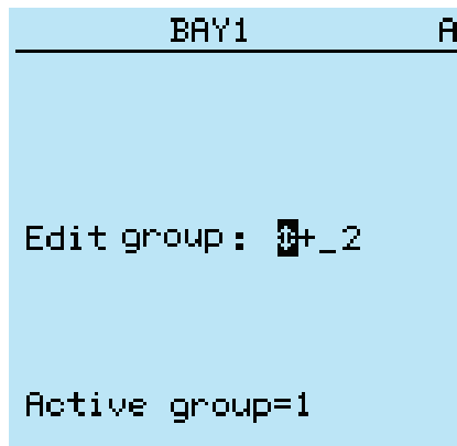
Figure 35: Restoring the previous value
