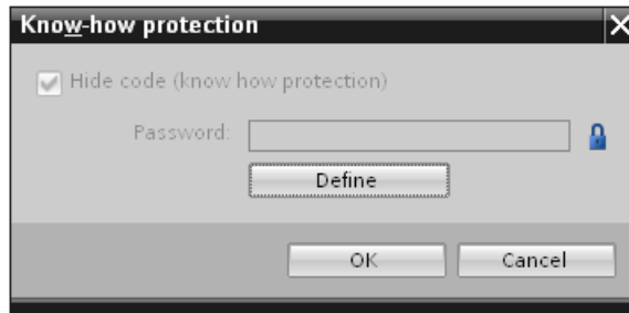
Figure 11-7 Setting up block know-how protection (2)
