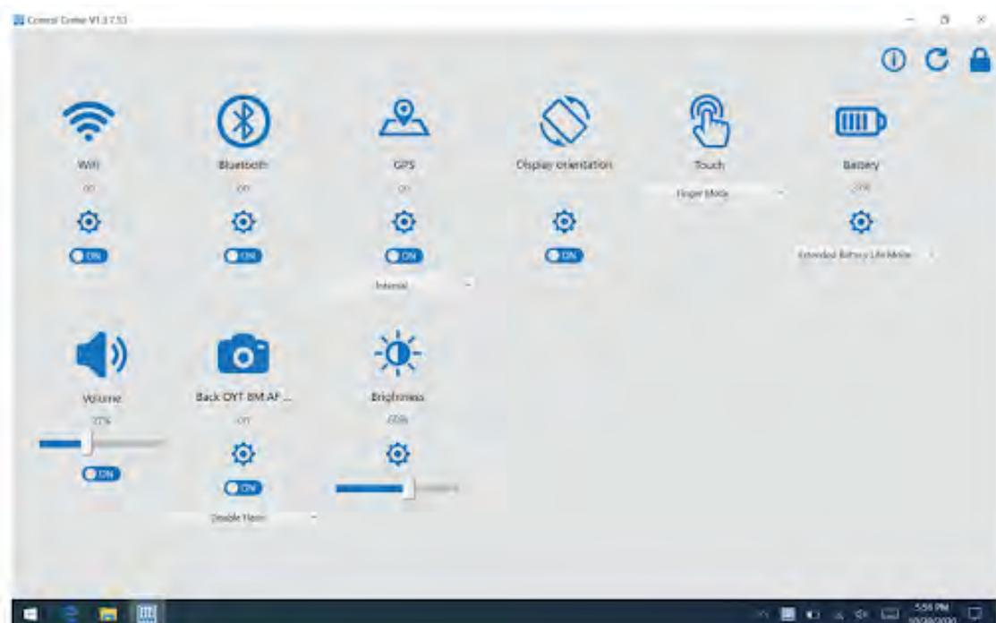
To access Authorized User Mode, click the lock icon on the top right corner of the application window. A dialog opens prompting the authorized user to enter the password. The default password is **DTRI**.
