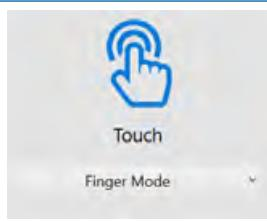
The drop-down menu allows you to quickly select the screen sensitivity. It supports Finger Mode, Glove Mode, and Water Mode.
