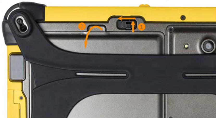
3. Insert a charged battery pack into the battery cavity—insert the bottom of the battery first to allow the battery tongues to seat correctly.
