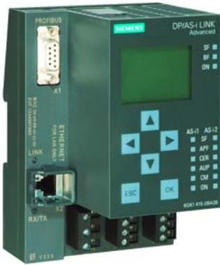
SIMATIC NET, DP/AS-Interface Link advanced, Gateway PROFIBUS DP/AS-Interface with master profile M3, M4 according to AS-i specification V3.0 for integration in PROFIBUS DP, Double master with display, Degree of protection IP20
