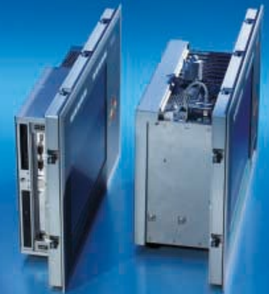
Panel PC = built-in Control Panel + add-on PC
