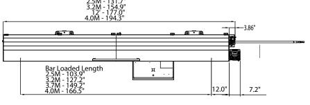
Barstock Straightness Specifications and Performance For optimum rotational performance speeds, bar stock straightness needs to be .020" per 3.25 feet, non accumulative. Bar stock out of this tolerance will not run at optimum RPM. Other factors such as material type (brass, copper, bronze and other malleable materials), clamping efficiency of the machine workholding, alignment of the bar feed, oil type, bar preparation and spindle liners will affect optimum RPM capability of the system.
