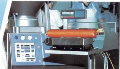
The MC control portions from 5 to 100,000 grammes. It is possible to set the desired weight with accuracy and the precision portioning system with a capacity of up to 500 portions/minute at 2.5 twists per link could scarcely be bettered.
