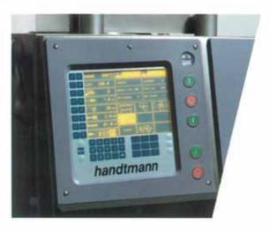
All VF 300 vacuum fillers can be equipped with Monitor Control, which is available on request. The operator is guided by screen prompts and, in addition to making inputs, can store product data via the monitor's screen. Monitor Control offers the operator a variety of information and allows flexible input and output of product data. In addition, product information can be stored, product names can be assigned, incorrect system operation is indicated in the display, etc.
