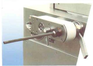
The linking gearbox type 34-4 is easily attached above the worktable. Its rapid coupling secures it firmly to the filler, whilst at the same time the linking gearbox automatically connects with the linking drive. Alignment and tools are not needed.
