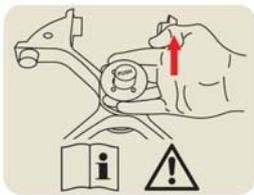
This Symbol refers to check, if the rotor is installed correct by lifting it slightly at the handle. See “[Rotor Installation](#)” on [page 31](#).
