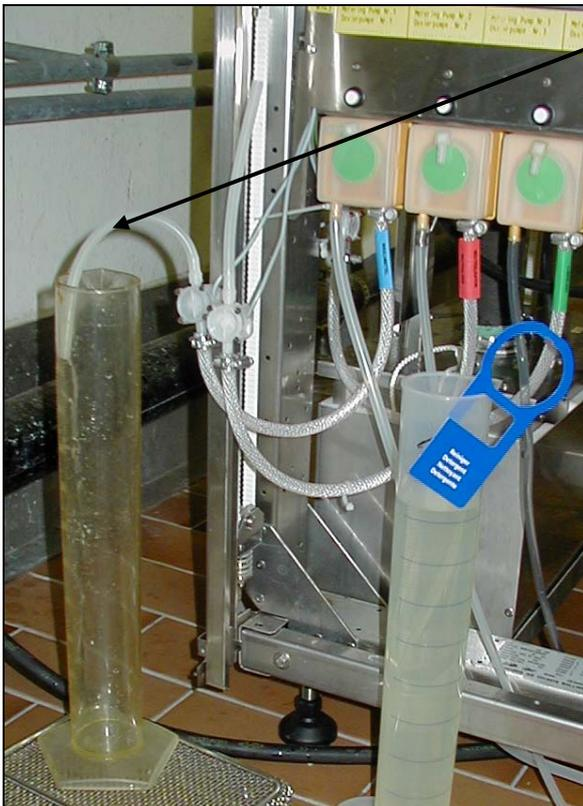
Remove hose from respective agent container elbow and place in calibration container (1 liter).
