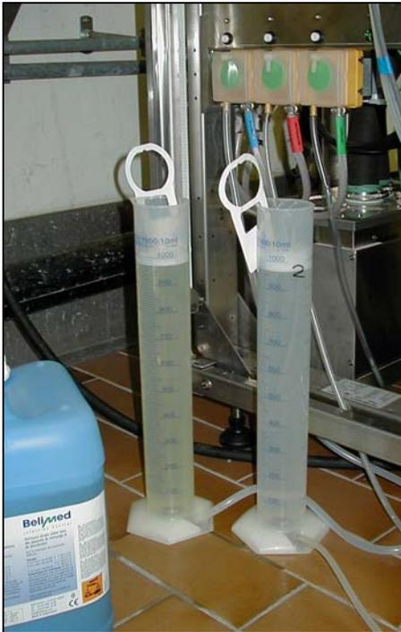
1. Remove hose from respective agent container elbow and place in measuring container (more than 1 liter).
