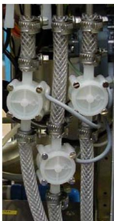
Check dosing system for leaks and accuracy. *The dosing hoses should be replaced at each service cycle.* Check connection elbows of wash chamber for leaks and hose connections for clamping torque of clamps. At each maintenance cycle or replacement of a safety related component, system needs to be recalibrated.
