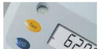
The level indicator is positioned directly next to the display for fast and easy levelling.
