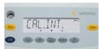
All BSA-CW balances come standard with an internal, motorized calibration and adjustment weight. Just touch the CAL key, and the balance will calibrate and adjust automatically.
