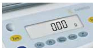
The new top-end models of the BSA precision balances deliver outstanding price | performance, with weighing ranges of 1 mg to 620 g and 10 mg to 6,200 g.
