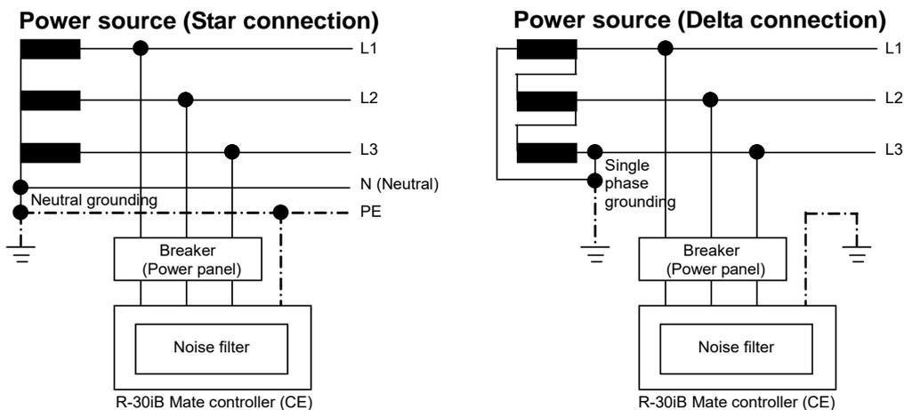
NOTE.2) R-30iB Mate/ R-30iB Mate Plus controller (CE) has a noise filter with switch that connect/disconnect the internal capacitor to the ground. In case that the controller connected to delta connection / single-phase grounding power system (TT-power system), it is possible to reduce the leakage current to less than 10mA by turning off (O-side) the switch at the noise filter.
