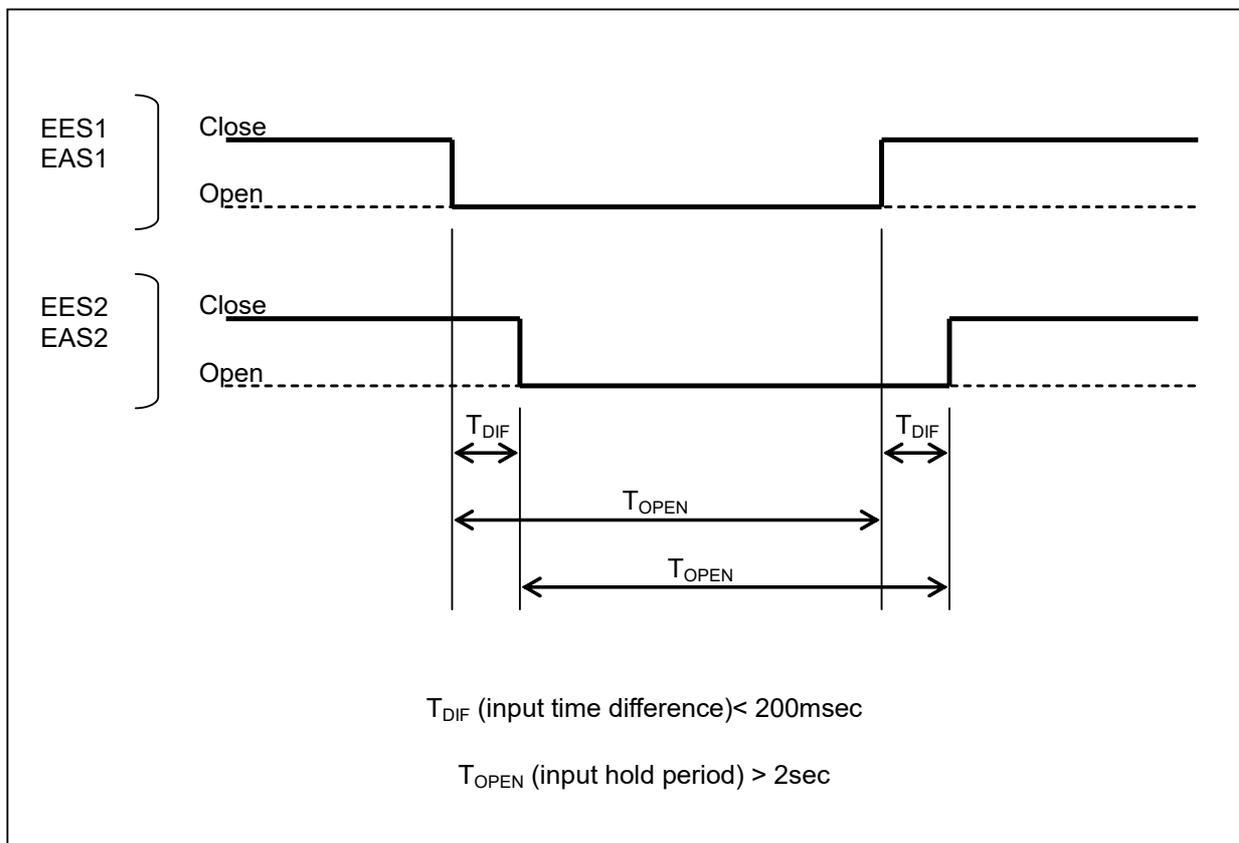
**Fig.3.3.4(c) Input timing of duplicate safety signals**
