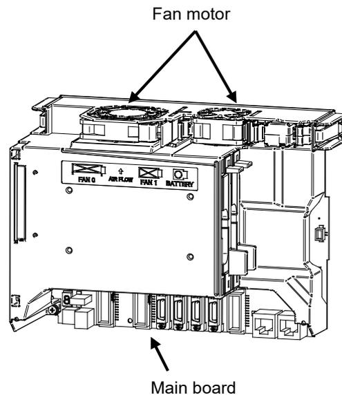
**Fig.3.5 (t) SRVO-123 Fan motor rev slow down(i)**
