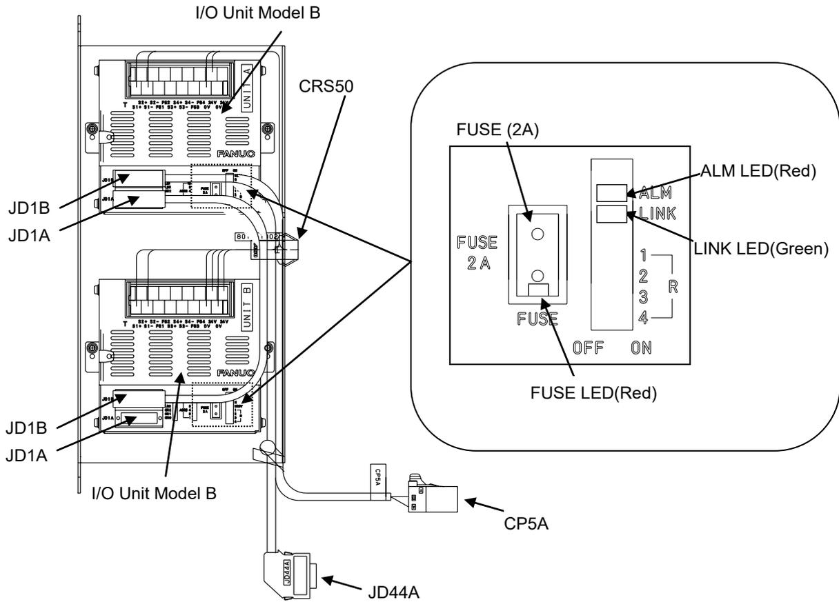
Fig.6 Sensor I/F unit for CR-4iA, CR-7iA
