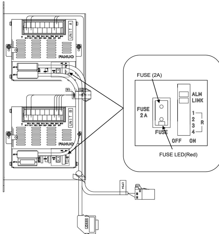
Fig.3.6 (f) Fuse on sensor I/F unit for CR-4*i*A, CR-7*i*A
