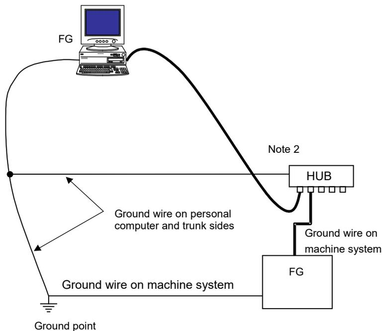
**Wiring on a single ground point**
