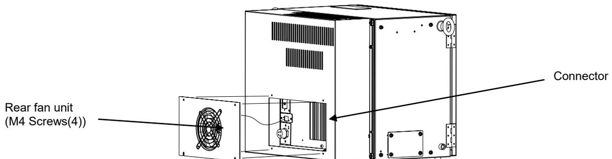
Fig.8.10.1(b) Replacing the rear fan unit
