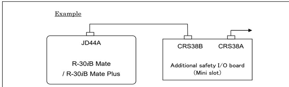
Fig.3.2.2 Connection of JD44A connector
