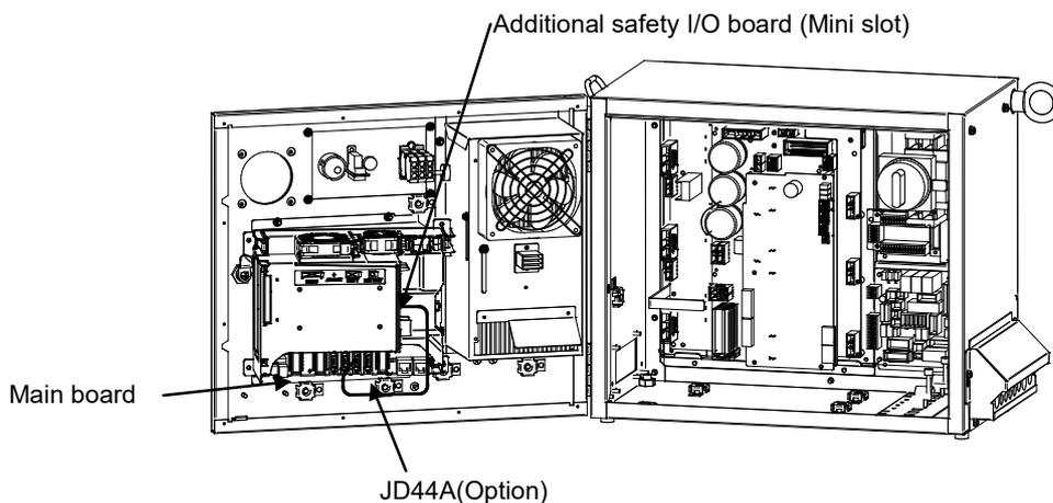
Fig.3.2.2.1 Path of the I/O link cable by using JD44A connector
