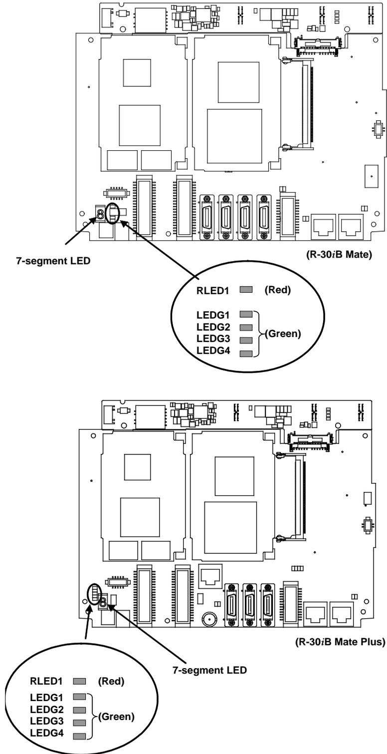
Fig. 3.7.1 Troubleshooting Using the LEDs On the Main Board
