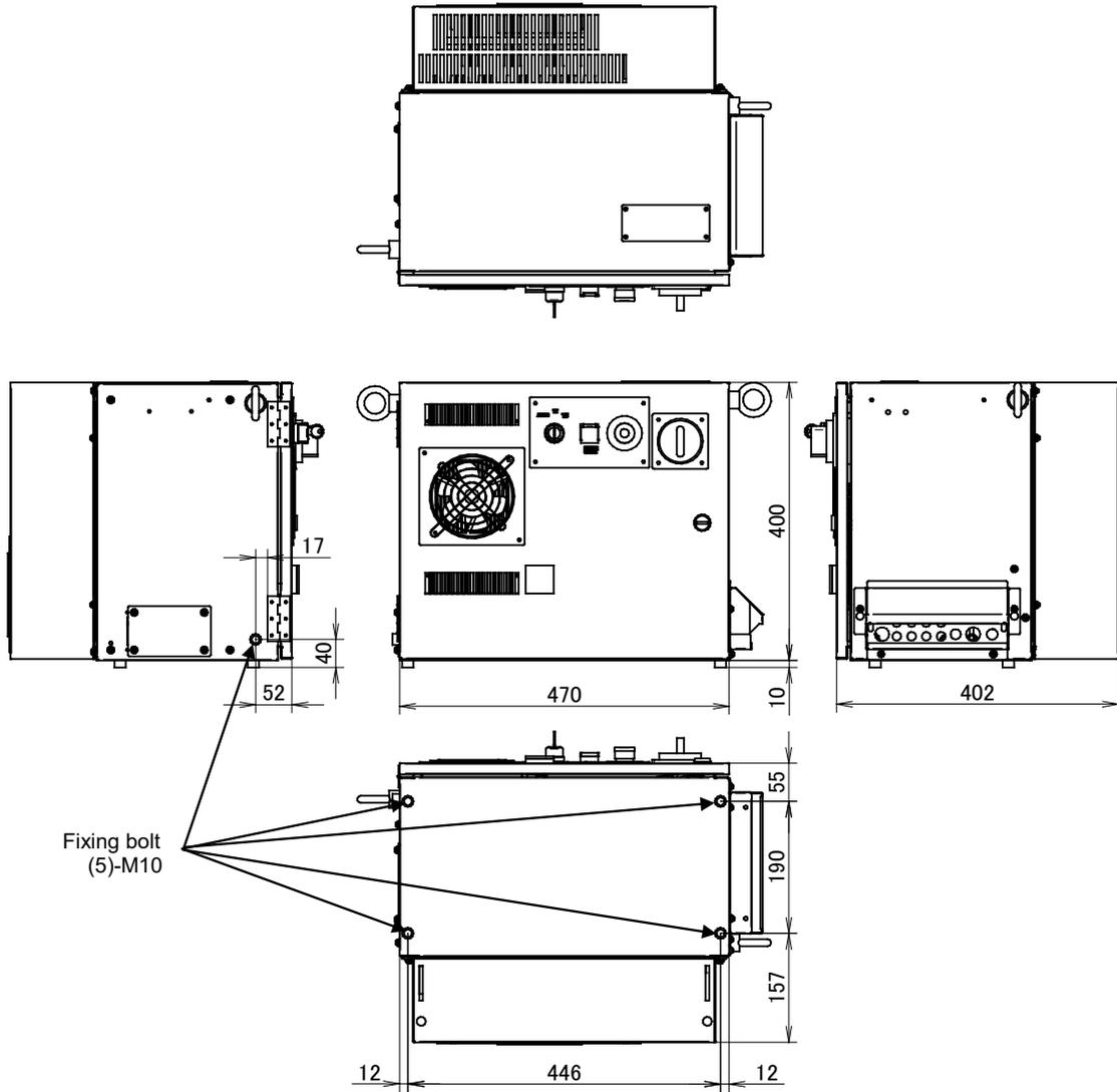
Fig.5.2.1(b) External dimensions (Medium / Large size)
