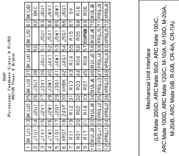
Fig.B(ac) Mechanical unit interface
