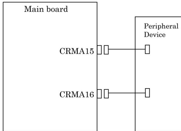
Fig.4.1.1 Block diagram of connecting peripheral device cable
