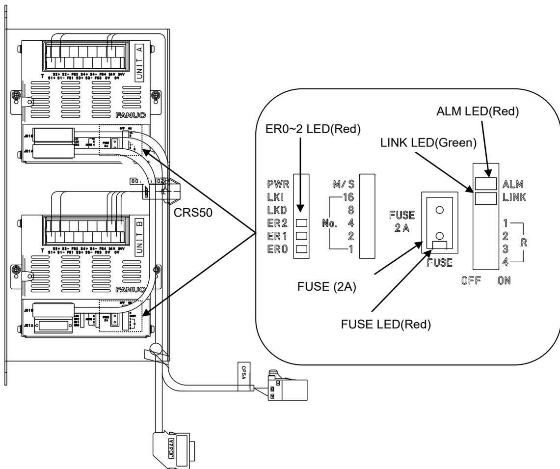
Fig.3.7.5 LEDs on the sensor I/F unit for CR-4*i*A, CR-7*i*A
