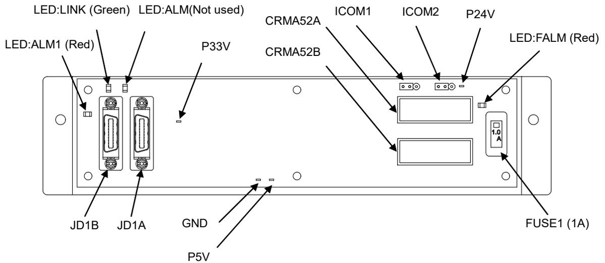
Fig.4.4 Process I/O Board MA
