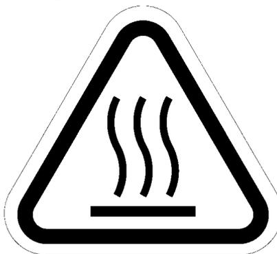
Fig.8 (b) High-Temperature warning label
