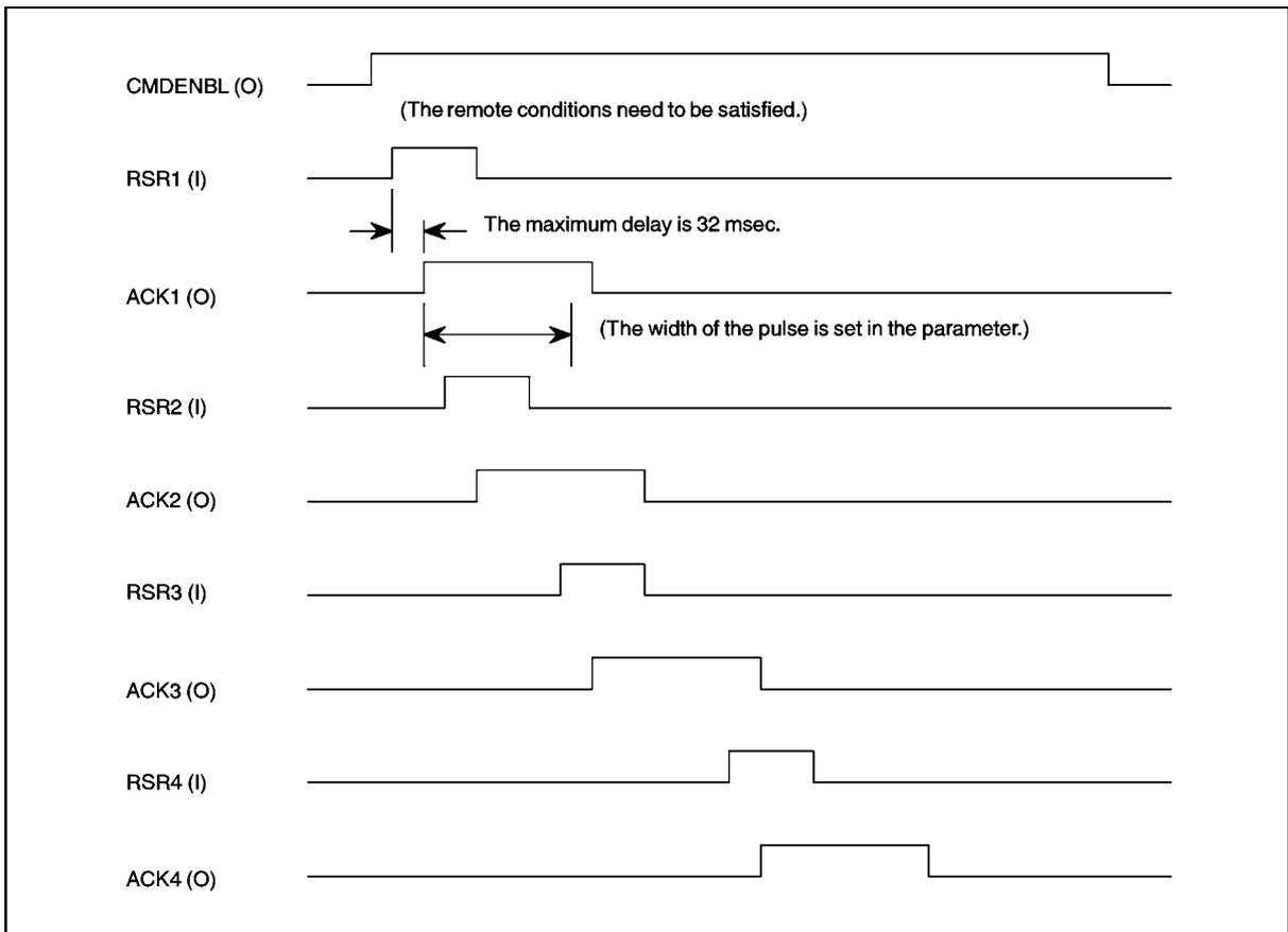
\* Other RSR signals can be accepted even when the ACK signal is being output.
