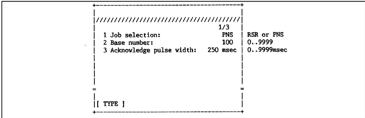
If a number other than zero is entered to PNS input, a program is selected whose program number is the entered value plus the base number. For example, if the PNS value is 23, the program to be started has the program name calculated from the expression
