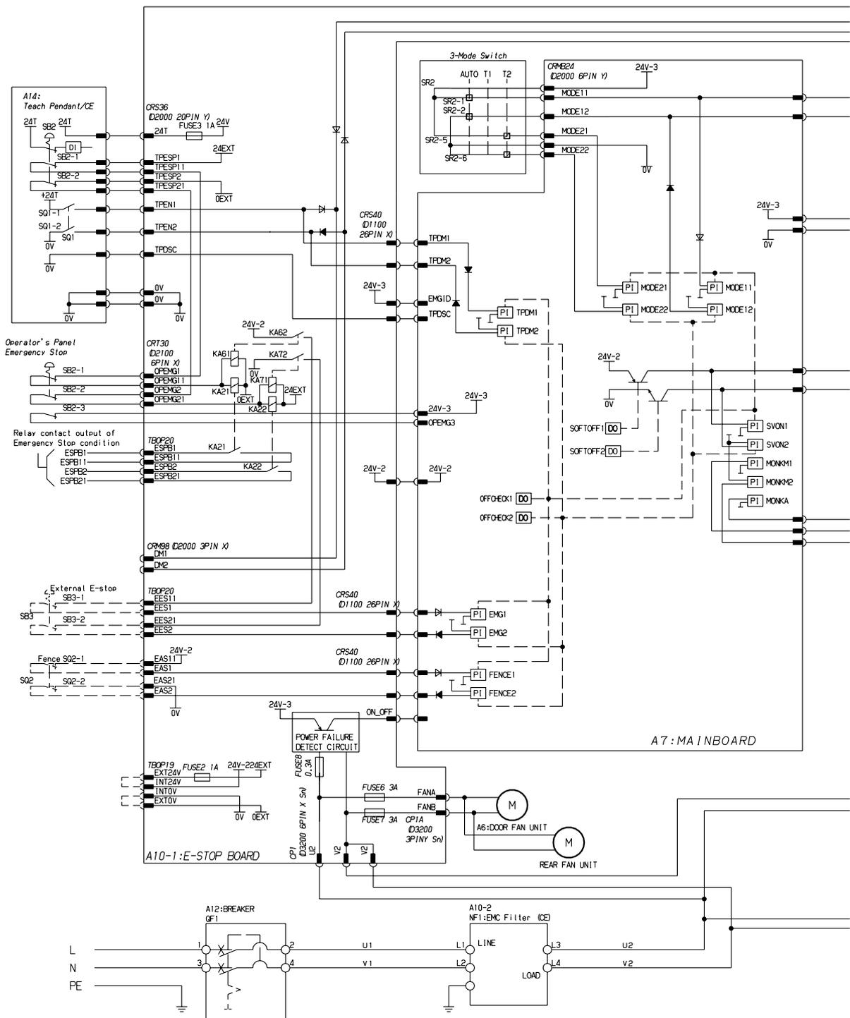
**Fig.B(j) R-30iB Mate Plus Emergency stop circuit connection diagram**
