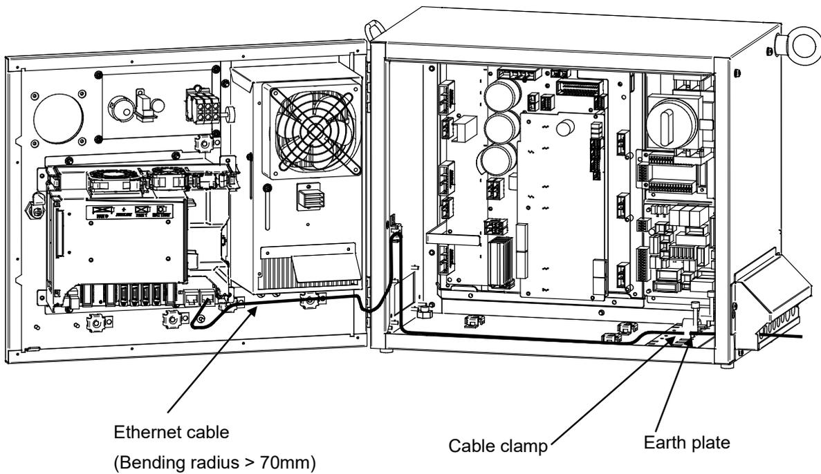
The Ethernet cable must be fastened by a cable clamp to prevent tension being applied to the modular connector (RJ-45) that connects the cable to the controller even if the Ethernet cable is pulled directly. This clamp is also used to ground the cable shield.
