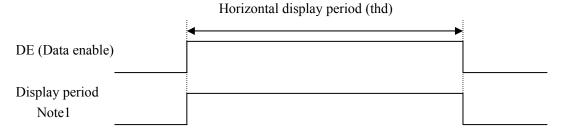
Note1: This diagram indicates virtual signal for set up to timing.
