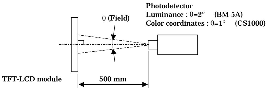
The luminance is measured according to FLAT PANEL DISPLAY MEASUREMENTS STANDARD (VESA Standard).
