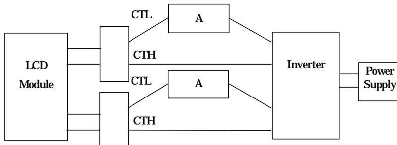
\*2) Lamp frequency of inverter may produce interference with horizontal synchronous frequency, and this may cause horizontal beat on the display. Therefore, please adjust lamp frequency, and keep inverter as far from module as possible or use electronic shielding between inverter and module to avoid the interference.
