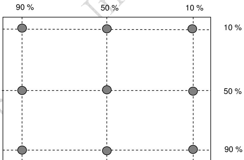
Note 3: The luminance uniformity of 9 points is defined by dividing the maximum luminance values by the minimum test point luminance
