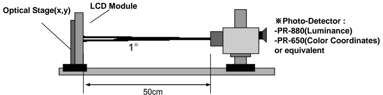
**FIG. 3 Electro-optical Characteristic Measurement Equipment and Method**
