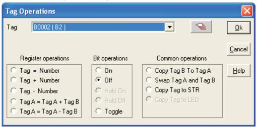
This task is executed on coil or bit-addressed register only. User can select coil or bit-addressed register from tag list. By using this task user can set bit/coil to 0.
