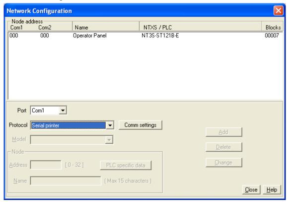
User can set either of the ports for serial printing. This is done by selecting Protocol as "Serial printer". In the above example, user has configured Com1 for serial printing. However, when this port is not being used for printing, it will be used for IBM Communication.
