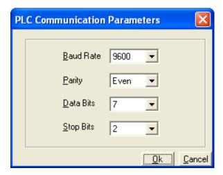
User can set PLC communication parameters like Baud Rate, Parity, Data Bits and Stop Bits. Click 'Ok' to set parameters.
