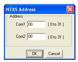
Note: Default Node address for unit is 0 for COM1 and COM2. This address needs to be changed if settings for PLC address is same as unit address.
