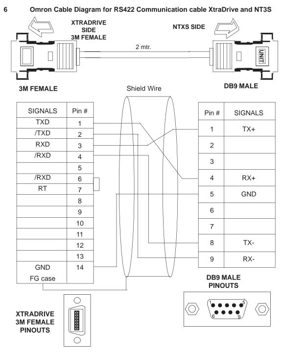
XtraDrive Connectro Type (3M) 10114-3000VE (Connector) 10314-52A0-008 (Cover)
