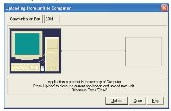
User can upload the application from the unit to the software from this dialog. Please check the unit and cable connections before starting upload.
