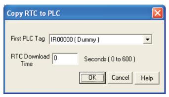
This task is supported only in Global task-list. This task copies sequentially 7 RTC parameters from selected tag after every specified RTC Download Time. If this time is specified as 0 sec. then it means this task will be executed as per Global task-list execution time.
