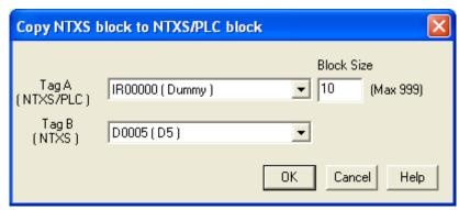
For e.g..- As shown above, 10 sequential unit tags starting from D0000 (i.e. D0000 to D0009) will be copied to 10 sequential PLC tags starting from IR00000 (i.e IR00000 to IR00009).
