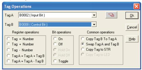
This task is executed on register tags and coil or bit-addressed register listed under Tag option. Both tag type must be of same type; either register type or coil/bit type. If the selected tags are of register type than this command is executed depending on the tag length (i.e. 1 byte,2 byte, 4 byte). User can interchange values of Tag A and Tag B by using this command.
