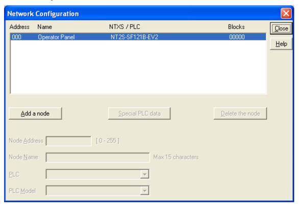
Node Address: User can assign unique node address starting from 0 to 255.
