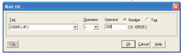
This task is supported only in 'While showing' Tasks of the Screen Tasklist . Tasks defined after this task are not executed until the condition specified is true.
