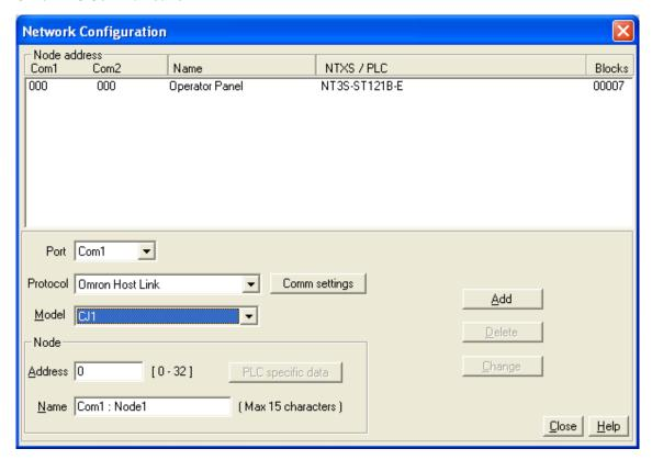
**Protocol** - User can select desired PLC from the list of available drivers. In the example shown above, user has selected Omron Host Link at Com1.
