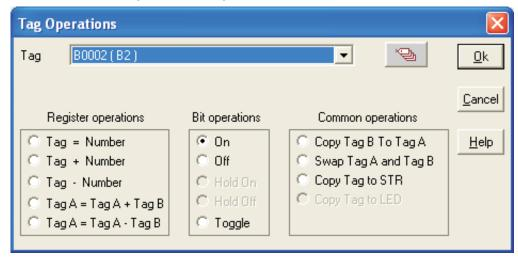
This task is executed on coil or bit-addressed register only. User can select coil or bit-addressed register from tag list.
