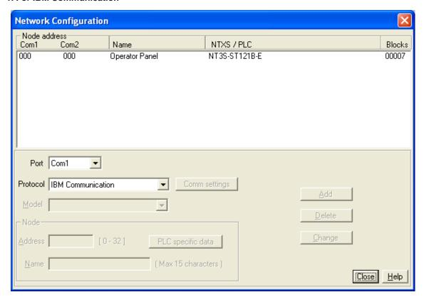
This is default communication setting. If user wants IBM communication, no other setting is required. In this case both communication ports can be used for download / upload purpose.
