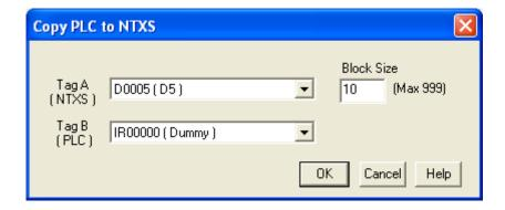
For e.g..- As shown above, 10 sequential PLC tags starting from IR00000 (i.e IR00000 to IR00009) will be copied to 10 sequential unit tags starting from D0000 (i.e. D0000 to D0009).
