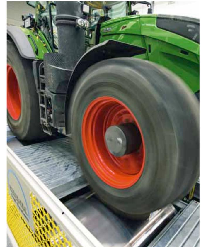
The distance between the axles can be adjusted from 2 – 6 m, which ensures that all tractors can be tested – from the 200 Vario to the 1000 Vario, and even more in the future.
