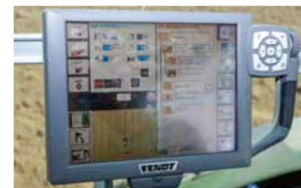
Fendt Terminal, VarioDoc, main page: The field to be worked and the waylines can be clearly recognised in the lower quarter of the terminal. The machine, operator, field, type of crop and the operation are documented on the right side in the main menu. After the work has been completed, the data are sent to the office computer.
