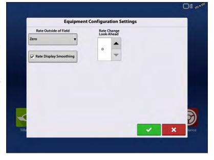
**Rate Change Look-Ahead**—This setting compensates for any latency in the control system when changing between different product rates during variable rate application. The typical setting range for this is 0-1 seconds. This setting can be thought of as a "look ahead" value when using a variable rate prescription. The display will send the signal to change rates before hitting a transition line so that the applied rate is correct when crossing into the new management zone.
