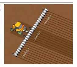
The system can be split between two channels to allow the down force to be adjusted separately on the planter wings and center section, where soil compaction is more likely to occur.
