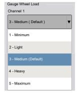
Wheel Load is defined as: The amount of gauge wheel load necessary to achieve proper depth 100% of the time, while minimizing compaction as much as possible (without risking loss of proper planting depth).
