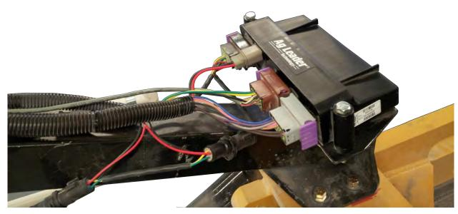
Make sure to color match the connections from the harness to the module and don't force the connections. This can prevent damage to electrical pins. The round connections on the harness are used to power the GPS receiver. The 3 large and 1 small square connections will connect to the module. The Brown connector will be used for the GPS signal input.
