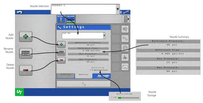
Creating nozzles is required for pressure based control, pressure fall-back, and droplet size monitoring. A nozzle's specifications are needed to achieve each feature.
