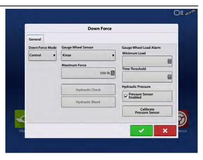
**Maximum Force**—used to limit the down force created by the actuator.
