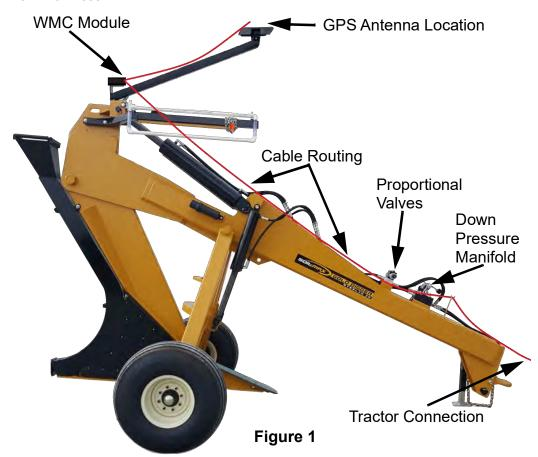
Locate cable PN 4003415. This will be mounted on the plow, with the single round cable connector at the hitch. There are 2 weather pack connectors that will connect to the proportional valve. Route the cable as shown below to ensure that moving parts do not pinch cables, extensions, or adapters.
