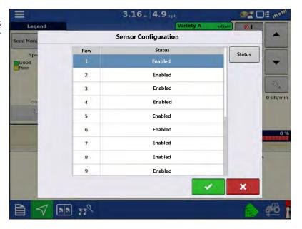
**Vacuum & Pressure Configuration**—If Air Seed Delivery or row Vacuum sensors are installed, you must configure them from this screen. Highlight the appropriate Row, then press **Install**. (This will also calibrate the vacuum sensor. Be sure to have the vacuum systems turned OFF.)
