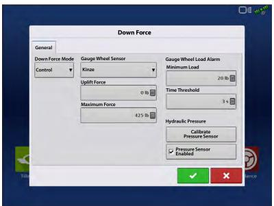
**Uplift Force**—usually 0 unless planter is equipped with uplift springs to provide an upward force on row units.
