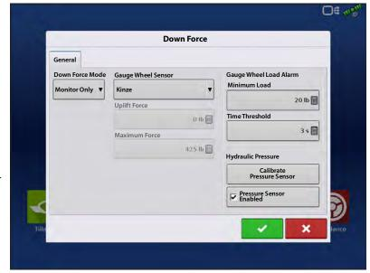
**Control mode**—as the planter travels across the field and encounters varying soil conditions (soil types, compaction zones, levels of debris) the display makes adjustments to the down force actuators on the row units, according to the gauge wheel load and the operator's settings, to maintain the correct seed placement in the soil.
