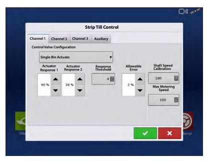
settings at the default value and making a small adjustment to this setting is usually all that is required to fine-tune system performance. The default setting is 4.
