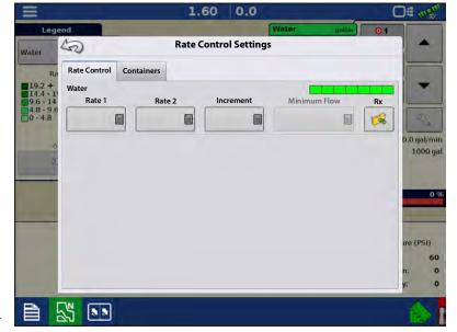
**Minimum Flow** — (Used for DirectCommand Liquid Applications only). This setting is used to maintain a consistent spray pattern. The display will not allow flow to drop below the entered setting. Set to flow at the lowest operating pressure for the selected spray tips with all sections on. When spraying with one or more boom sections off, the system automatically reduces the Minimum Flow setting according to the reduced spray width. To adjust this setting, press the desired numeric value.
