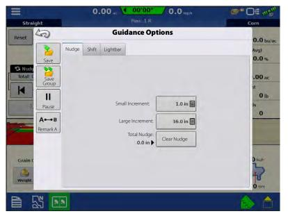
Shift moves all of the swaths by a specified distance to the left or right, (including the AB line). The swaths can be shifted by a distance or number of rows.
