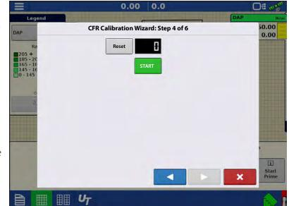
2. **Enter Actual Weight**—The Accumulated Weight is shown in the top portion of the screen. Press to enter the Actual Weight applied, and press to continue.
