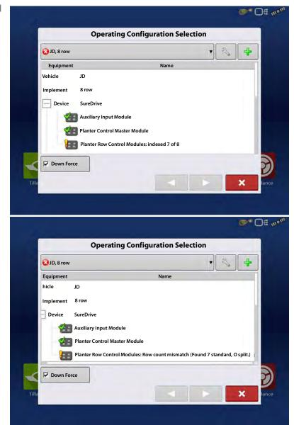
Image 2 - The message that will appear when there are more modules on the CAN bus than what the config requires.
