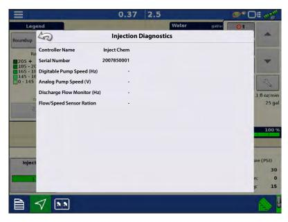
• Flow/Speed Sensor Ratio—The ratio that the system derived for calibration.
