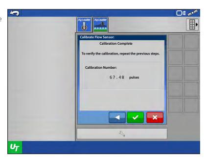
This method will use the sprayer to dispense a known amount of liquid. Please use water to calibrate when using this method.
