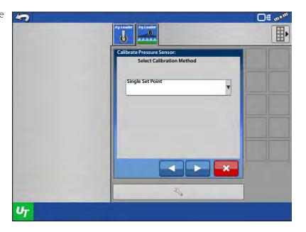
2. Enter the mV/psi calibration value of the sensor. A sensor provided by Ag Leader is 16 mV/psi. If the calibration number of the sensor is unknown, press
