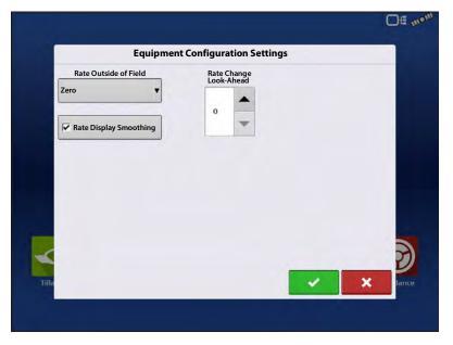
**Rate Change Look-Ahead**—This setting compensates for any latency in the control system when changing between different product flow rates during variable rate application. The typical setting range for this is 0-1 seconds. This setting can be thought of as a "look ahead" value when using a variable rate prescription. The display will send the signal to change rates before hitting a transition line so that the applied rate is correct when crossing into the new management zone.
