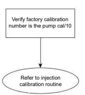
The injection module requires that a pump calibration be performed before actual application can occur. The calibration number found on the tag of the injection pump's digital speed sensor needs to be divided by a factor of 10 before entering it as the factory calibration number. If the factory cal number is entered wrong, the pump calibration routine will not finish due to a high application error.
