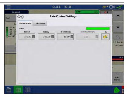
**Minimum Flow** — (Used for DirectCommand Liquid Applications only). This setting is used to maintain a consistent spray pattern. The display will not allow flow to drop below the entered setting. Set to flow at the lowest operating pressure for the selected spray tips with all sections on. When spraying with one or more boom sections off, the system automatically
