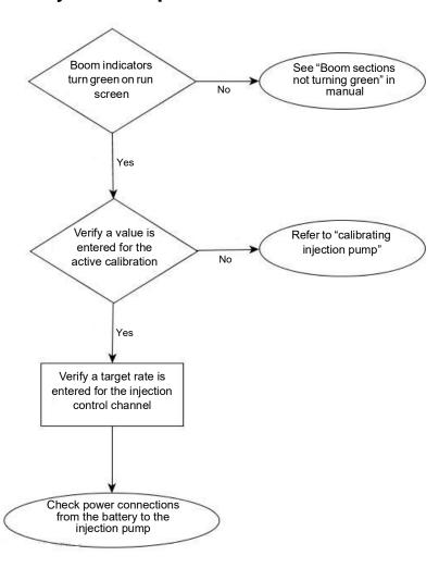
Power can be checked at multiple locations. First is the connection at the Injection module where the battery power cable plugs in. The second location is the output connection found on the injection module. The third is found at the 2 pin weather-pack tower found on the injection cable PN: 4000851-3. See table below.
