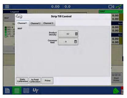
**In-Field Calibration**—Press the In-Field Calibration button to perform an automated routine to adjust the calibration number for the selected metering circuit. This calibration is performed if there is a difference between the amount of product logged as compared to what was actually applied. For more information, see "In-Field Calibration Procedure" on page 598.
