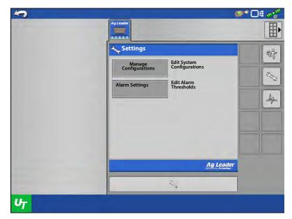
**Warning Enabled** – With this setting enabled, the user will get a "Rate Not Responding" alarm when the actual rate does not fall within the threshold and timeout settings. The user will not receive an alarm if this setting is disabled.
