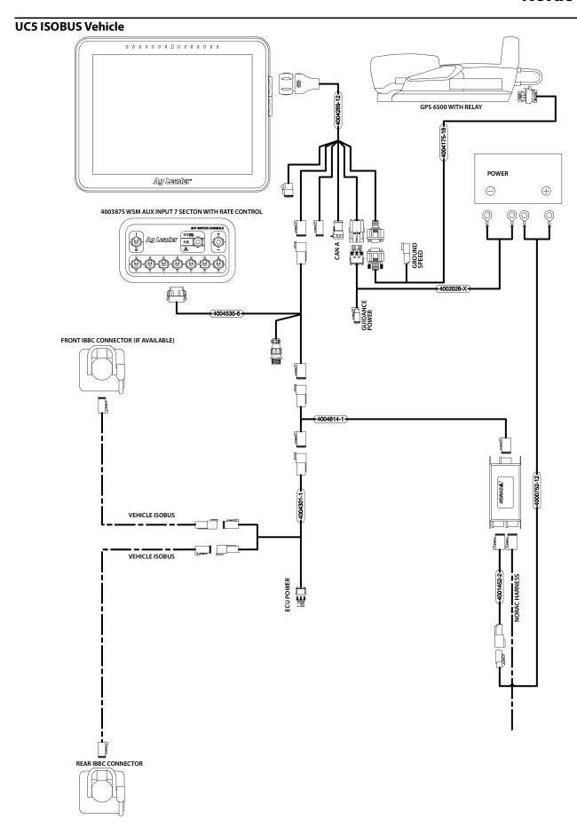
DirectCommand<sup>™</sup> for spinner spreaders is capable of controlling the product conveyor, spinner speed, monitoring bin level, and providing multiple prescription rate control for up to five granular products. The control modules support PWM, motorized servo, Mark IV.2, Mark IV.4, and Mark V hydraulic control valves. DirectC+ommand granular application system also supports application control of multiple bin spreaders.
