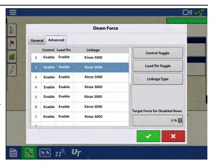
**Linkage Type** — This allows the operator to change the row unit Linkage Type. Planters may have a combination of short and long parallel arms. Linkage type can be selected independently for each row. Multiple rows can be selected together when changing the Linkage Type.
