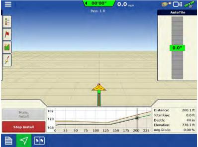
To extract the plow, press the "Up" button to manually nose the plow up while pulling ahead to bring the plow out of the ground.
