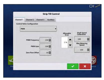
**Allowable Error**—Determines the percent of error that is allowed prior to the product control system making any flow rate changes. 2% - 3% is the normal dead band setting range.
