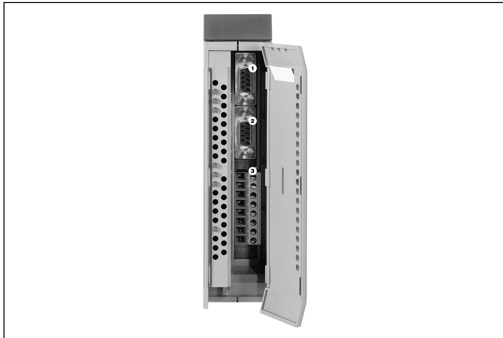
Figure 197: NC150 operational and connection elements
