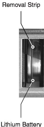
Figure 61: CP340, CP360, CP380 and CP382 - removal strip should be pulled to the right
