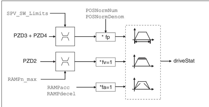
Figure 8.11 Profile position operating mode, effect of settable parameters
