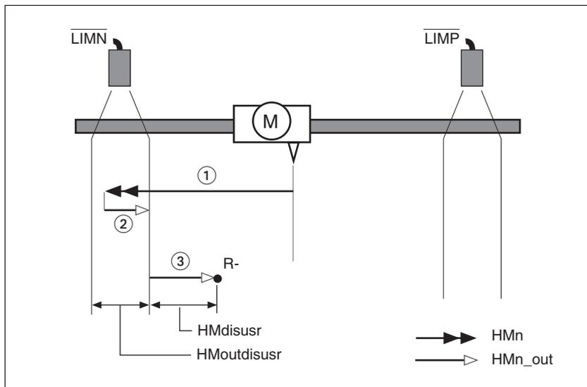
Figure 8.13 Reference movement to the negative limit switch
