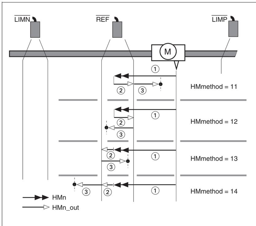
Figure 8.17 Reference movements to the reference switch
