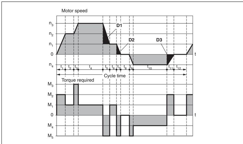
Figure 6.10 Characteristics for rating the braking resistor
