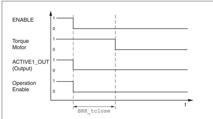
Figure 8.29 Applying the holding brake
