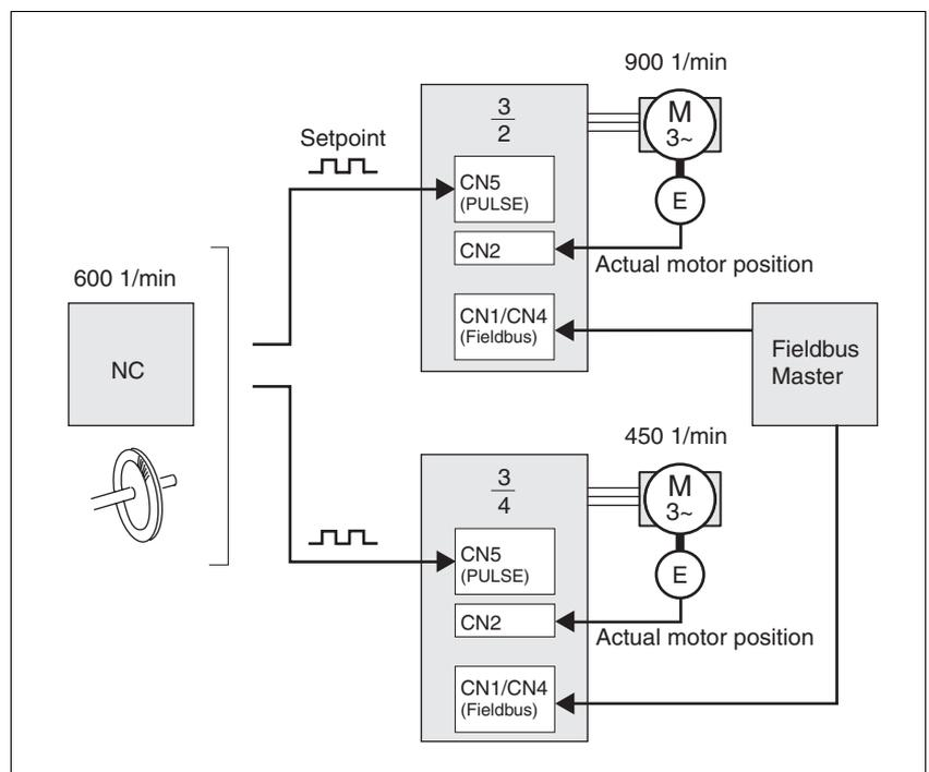
Figure 8.8 Reference value preset via NC controller
