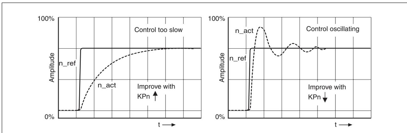
Figure 7.13 Optimise inadequate settings of the speed regulator
