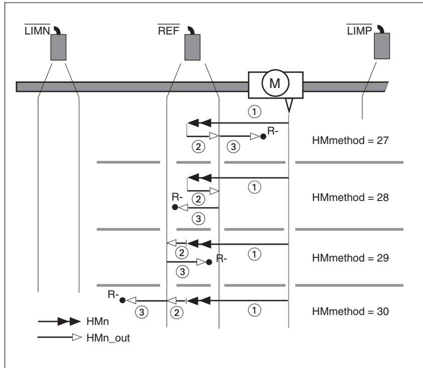
Figure 8.14 Reference movements to the reference switch
