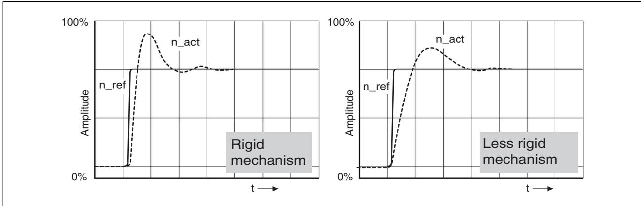
Figure 7.12 Step responses with good control behaviour
