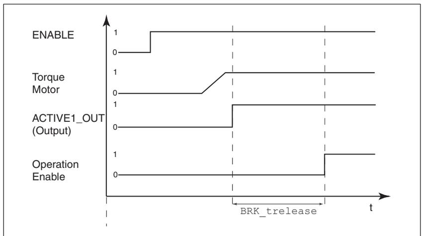
Figure 8.28 Releasing the holding brake
