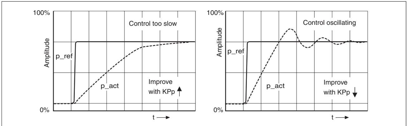
Figure 7.15 Optimising improper settings of the position controller
