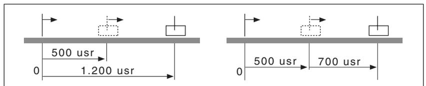
Figure 8.10 Absolute positioning (left) and relative positioning (right)
