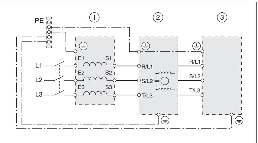
Figure 6.12 Wiring diagram: mains power for 3-phase device
