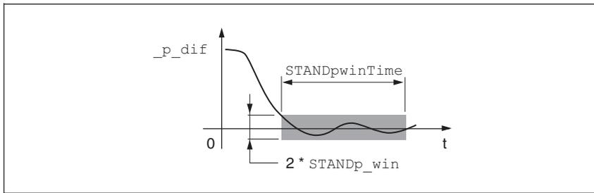
Figure 8.27 Standstill window
