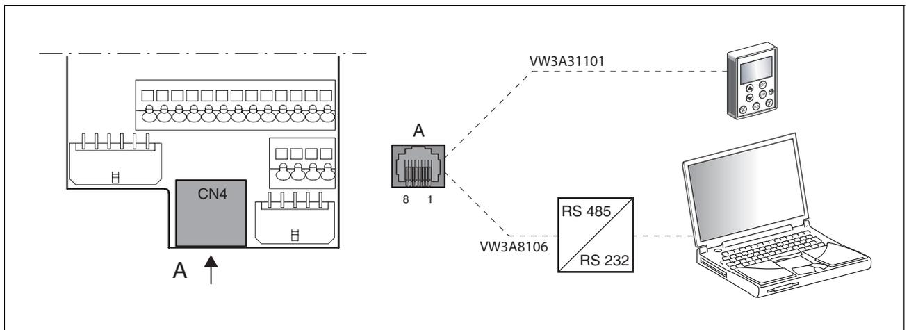
Figure 6.28 Wiring diagram of PC or remote terminal
