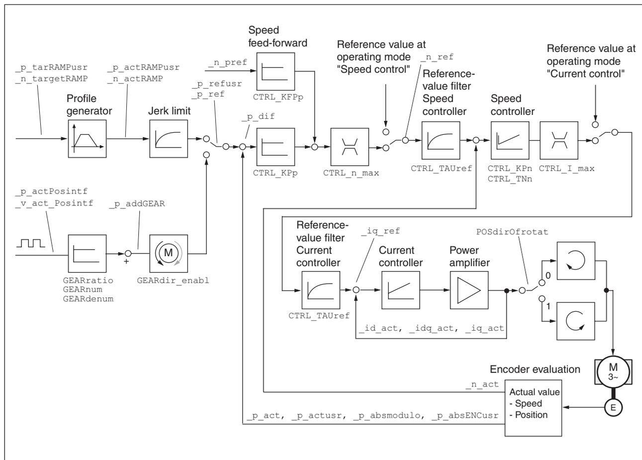
Figure 8.21 Status monitoring of the control loops
