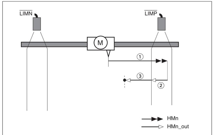
Figure 8.16 Reference movement to the positive limit switch
