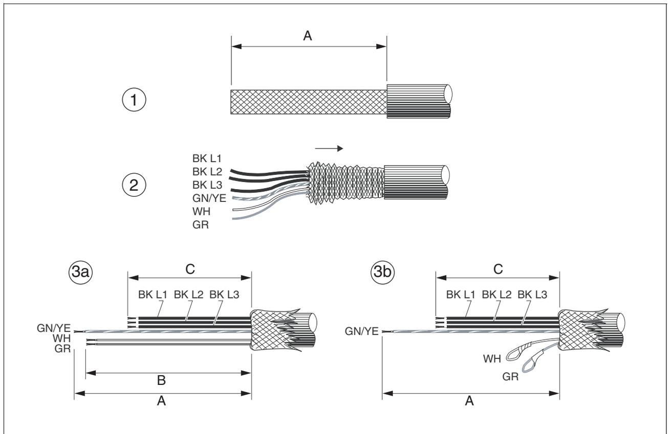
Figure 6.6 Steps (1-3) for fabrication of the motor cable
