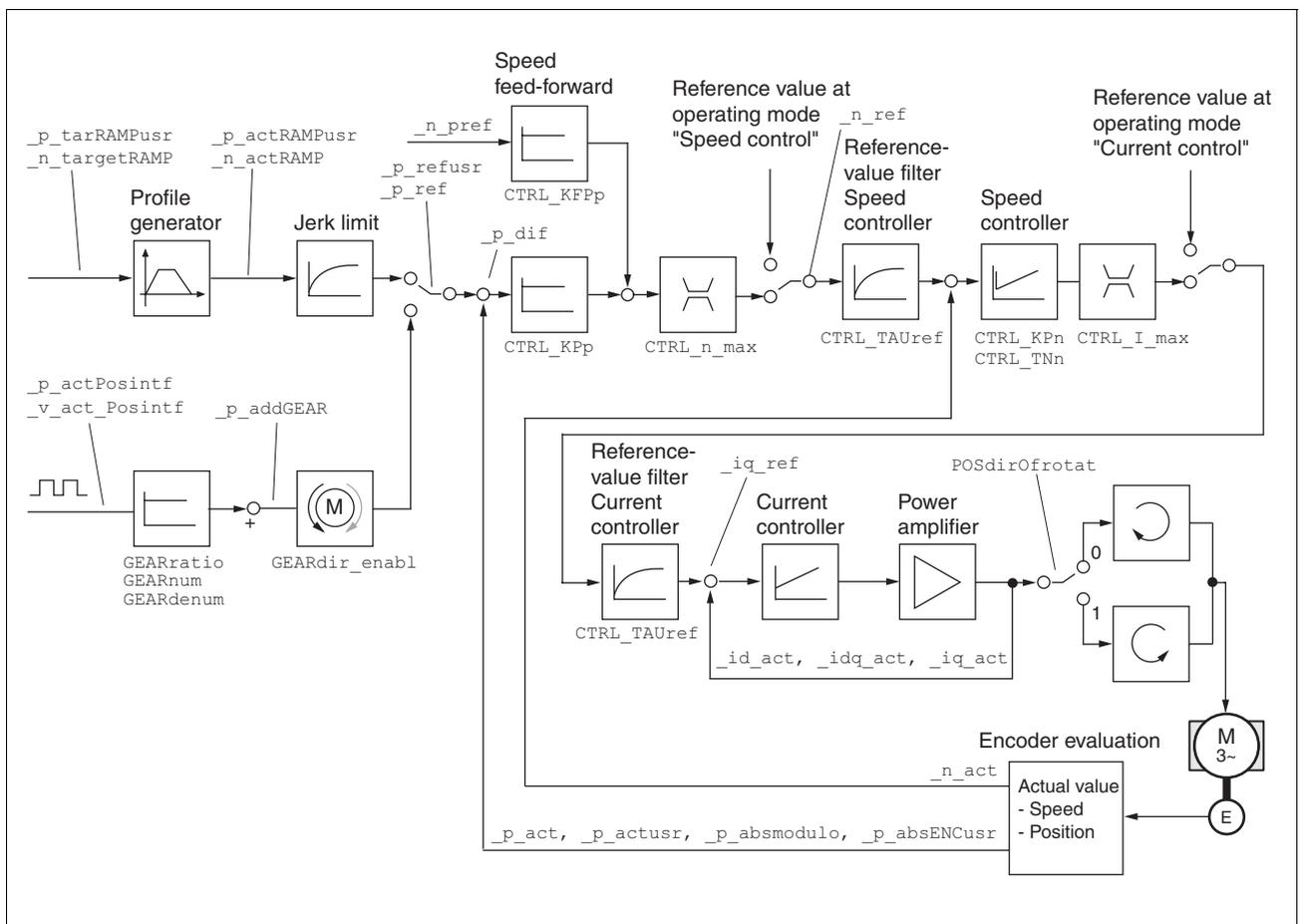
Figure 7.9 Controller structure for encoder evaluation via CN2
