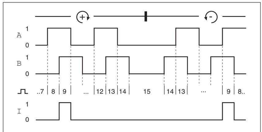
Figure 6.22 Timing diagram with A, B and index pulse signal, counting forwards and backwards
