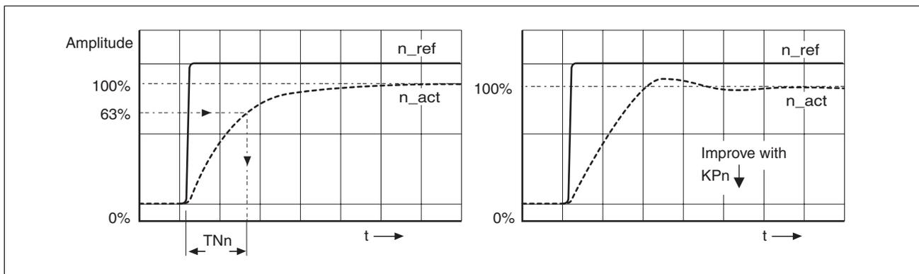
Figure 7.11 Determining 'TNn' in the aperiodic limiting case
