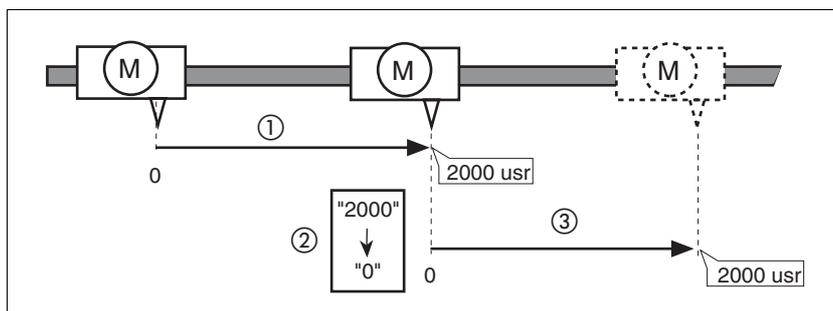
Figure 8.20 Positioning by 4000 usr units with dimension setting
