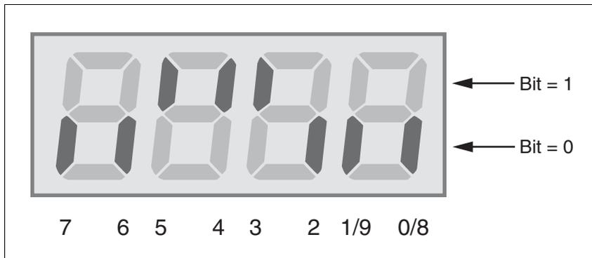
Figure 7.7 HMI, status display of the digital inputs/outputs
