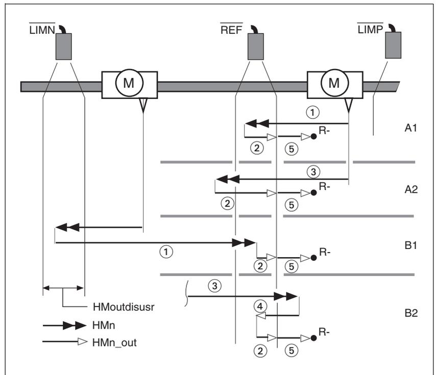
Figure 8.15 Reference movements to the reference switch
