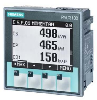
SENTRON PAC3100; LCD; 96X96MM POWER MONITORING DEVICE PANEL MOUNT TYPE FOR MEASUREMENT OF ELECTR. VALUES UC: 110-250VDC / 100-240VAC UE: MAX.480/277V; 45-65HZ IE: X/5A AC TERMINAL CONNECTION
