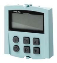
SIPLUS S120 BOP20 Basic Operator Panel -20...+70°C with conformal coating based on 6SL3055-0AA00-4BA0 . Actuator with miniature display 2-line, 6 keys for parameter assignment and diagnostics suitable for Control Units CU305, CU310, CU320
