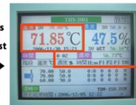
To assure the TDM can function properly in harsh working environment, the internal temperature of test chamber was set in the range -30°C to +70°C.
