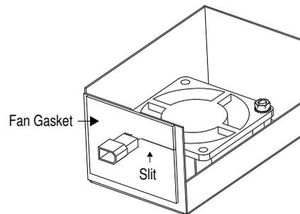
4. Press the gasket firmly to the fan housing to secure the gasket.
