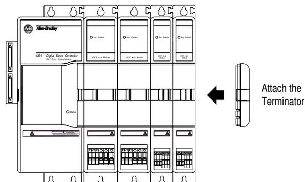
**Important:** The terminator terminates the serial ring and provides protection for the DC Link. The 1394 system will not operate without the terminator.
