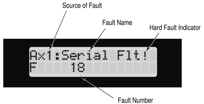
Each area on the diagram in Figure 9.1 has a significance:
