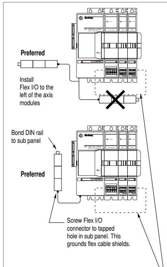
**Important:** You must separate low voltage I/O from all exposed high voltage conductors to avoid the affects of EMI and RFI.
