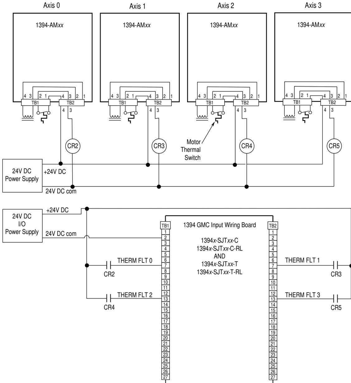
Note: 120V AC (50 or 60 Hz) power may be used in place of a 24V DC power supply for motor thermal switch circuits.
