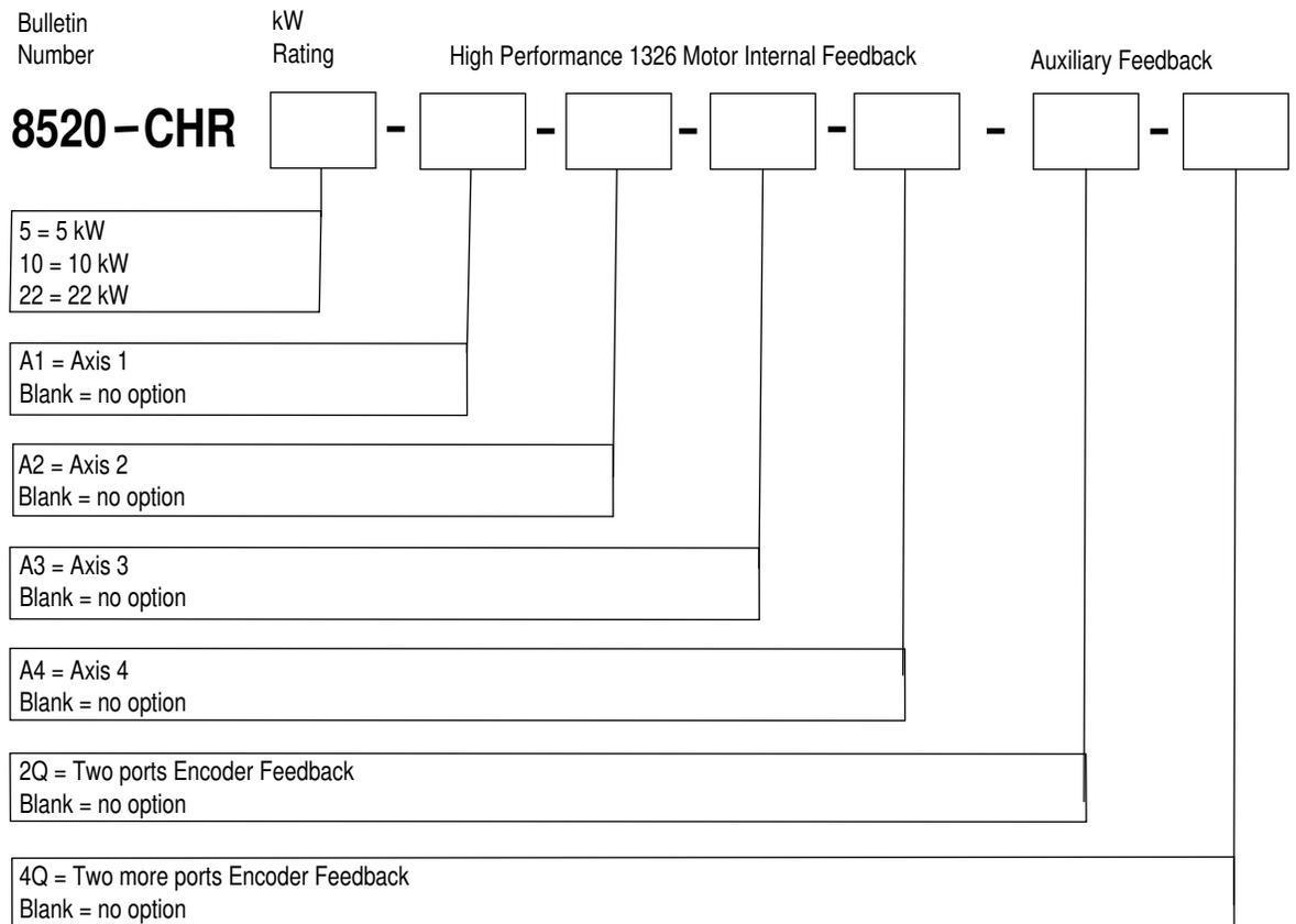
Note: 8520-CHR (Series C) system modules include Smart Power, improved terminations, and EMI filtering. Refer to *9/Series Integration and Maintenance Manual* (publication 8520-6.2) for more information.
