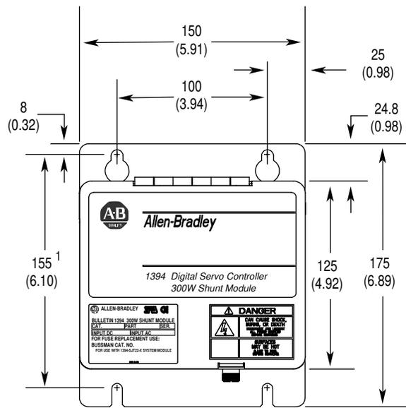
Dimensions are in millimeters and (inches)
