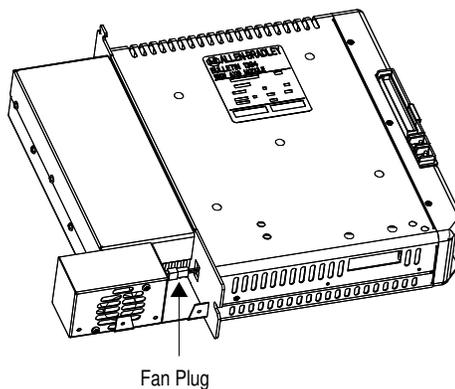
6. Unplug the fan housing from the axis module.
