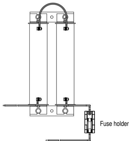
3. Remove the fuse from the fuse holder with the fuse puller tool.
