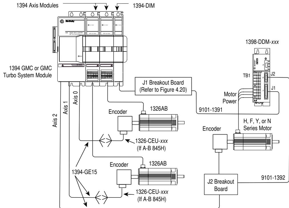
Figure 4.20 shows the J1 breakout board interconnect details between the 1394-DIM and the 1398-DDM-xxx. Refer to *ULTRA 200 User Manual* (publication 1398-5.0) and *ULTRA 100 User Manual* (publication 1398-5.2) for more information.
