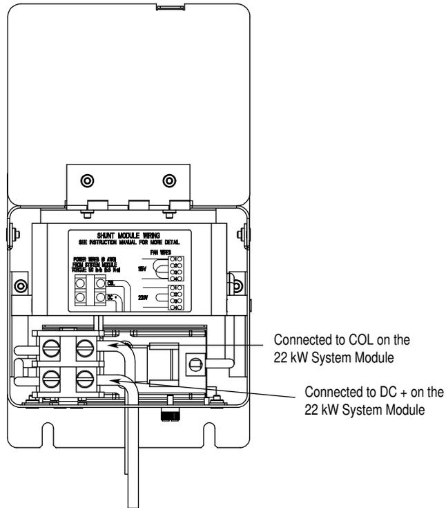
10. Tighten both screw terminals (torque = 2.5 N-m, 22.1 lb-in.).
