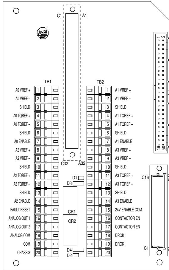
**Important:** Use the terminal operating tool (supplied with the system module) to help you insert and remove wires on the input wiring board.
