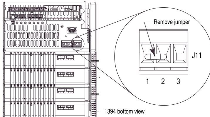
3. Install the shunt resistor wire leading to the fuse in connector J11-1.
