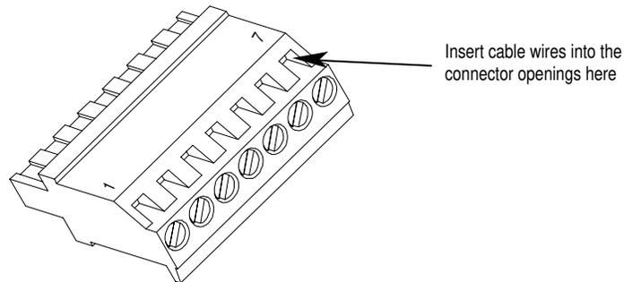
8. Use a screwdriver to tighten the clamping screw to the correct torque (0.25 N-m/2.2 lb-in.) until the cable lead cannot be pulled out of the terminal.
