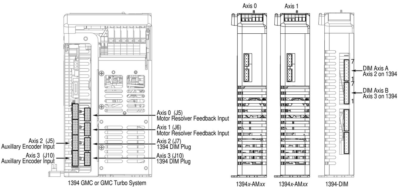
The example below shows one 1394 axis and one DIM output axis.
