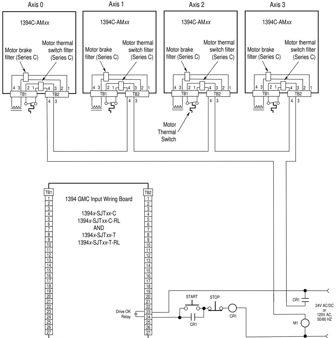
The example below shows 1394 (Series C) axis modules wired for thermal fault monitoring. Depending on how the 1394 GMC system is configured, the fault can be used to disable one or all of the four axis modules.
