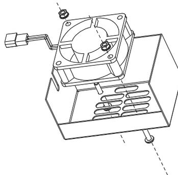
10. Remove the fan from the fan housing.
