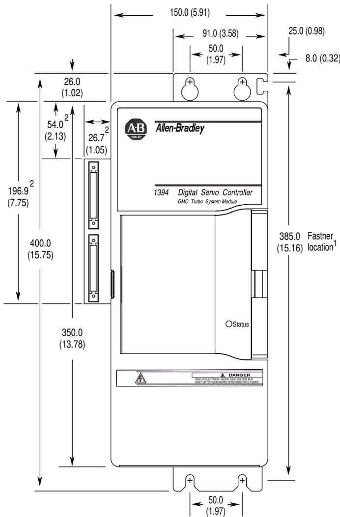
Dimensions are in millimeters and (inches)
