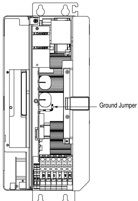
7. Without removing the circuit board, unplug the jumper and move it to the ungrounded power distribution position. Refer to the figure below for the jumper positions.
