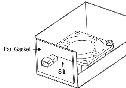
8. Remove the fan gasket from the fan housing. Make sure you slide the fan wires through the slit in the gasket.
