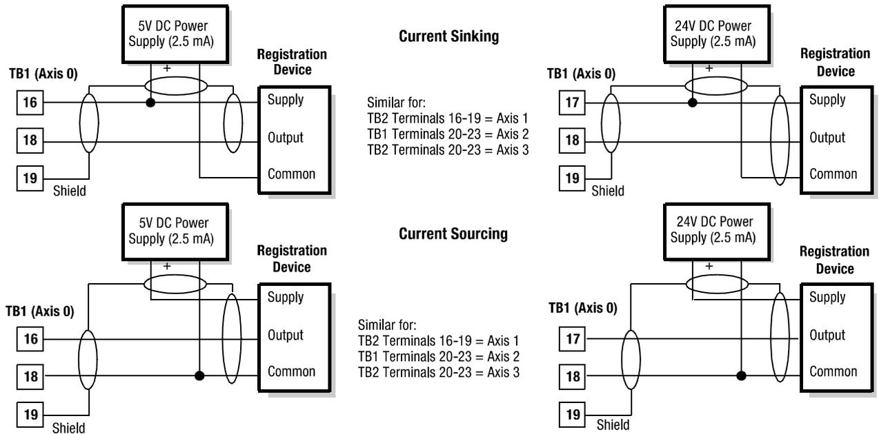
**Important:** Connections shown are typical only. Some input devices vary in their specific connections. Consult the wiring diagram for your device.
