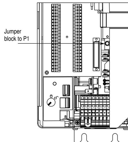
4. Install and tighten the resistor wire with the fuse in the DC+ terminal on the power terminal block in the lower right corner.
