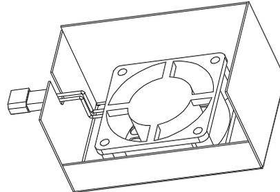
2. Peel the adhesive backing off of the new fan gasket.
