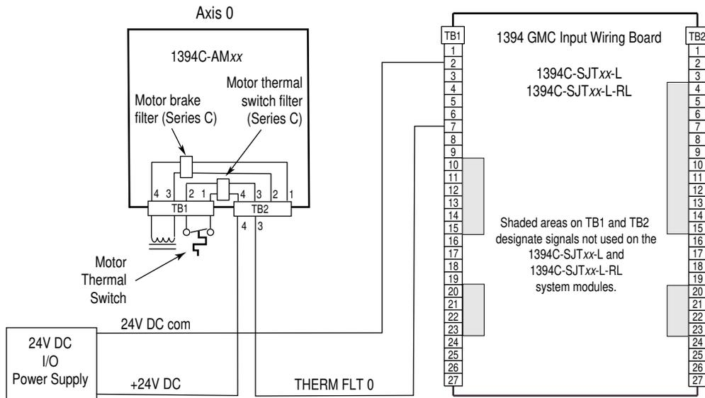
Note: 120V AC (50 or 60 Hz) power may be used in place of a 24V DC power supply for the motor thermal switch circuit.
