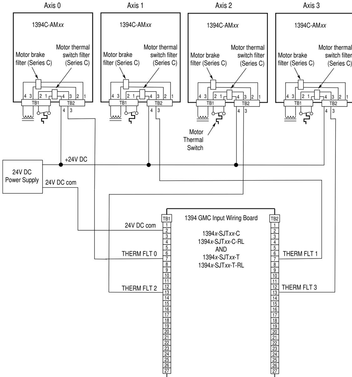
Note: 120V AC (50 or 60 Hz) power may be used in place of a 24V DC power supply for motor thermal switch circuits.
