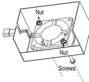
6. Align the fan housing to the axis module.
