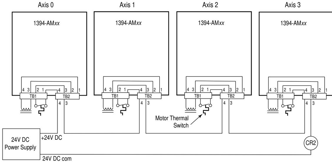
Note: 120V AC (50 or 60 Hz) power may be used in place of a 24V DC power supply for motor thermal switch circuits.
