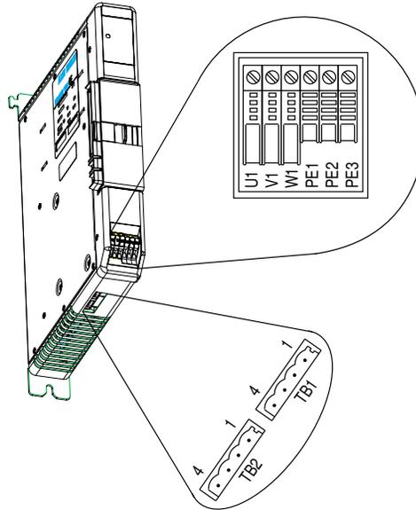
**Important:** Noise filters on the motor thermal sensor and brake connectors (TB1 and TB2) add capacitance ( $1.0 \mu\text{F}$ ) from each leg of the thermal switch and motor brake leads to ground. This should be considered when selecting ground fault circuits.
