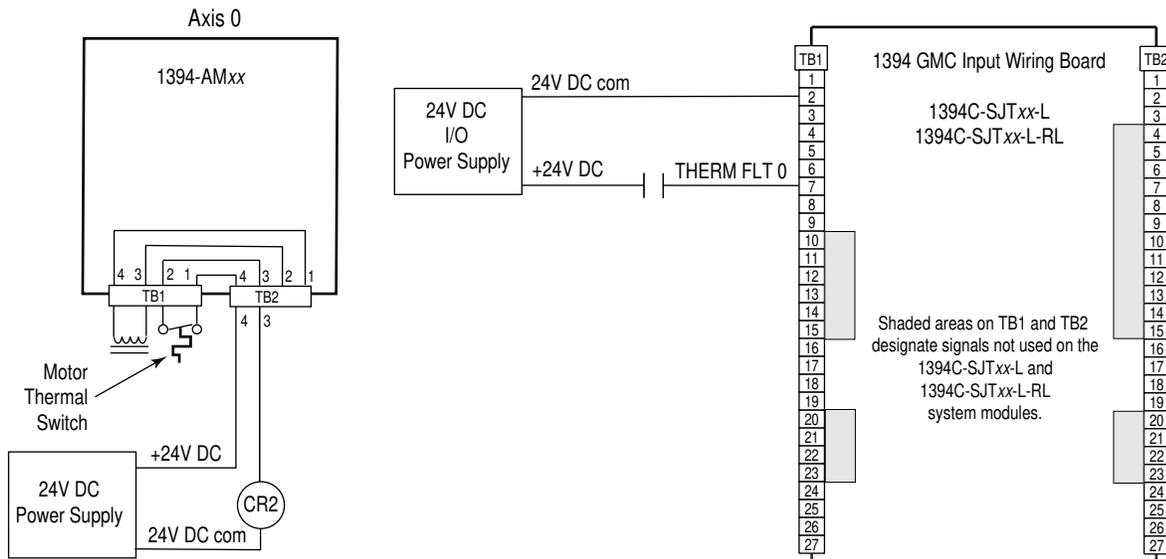
Note: 120V AC (50 or 60 Hz) power may be used in place of a 24V DC power supply for the motor thermal switch circuit.
