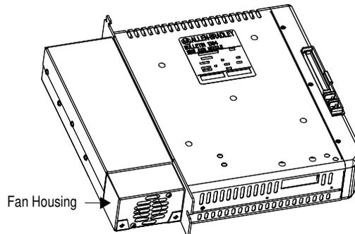
4. Remove the screws that hold the fan housing to the axis module.
