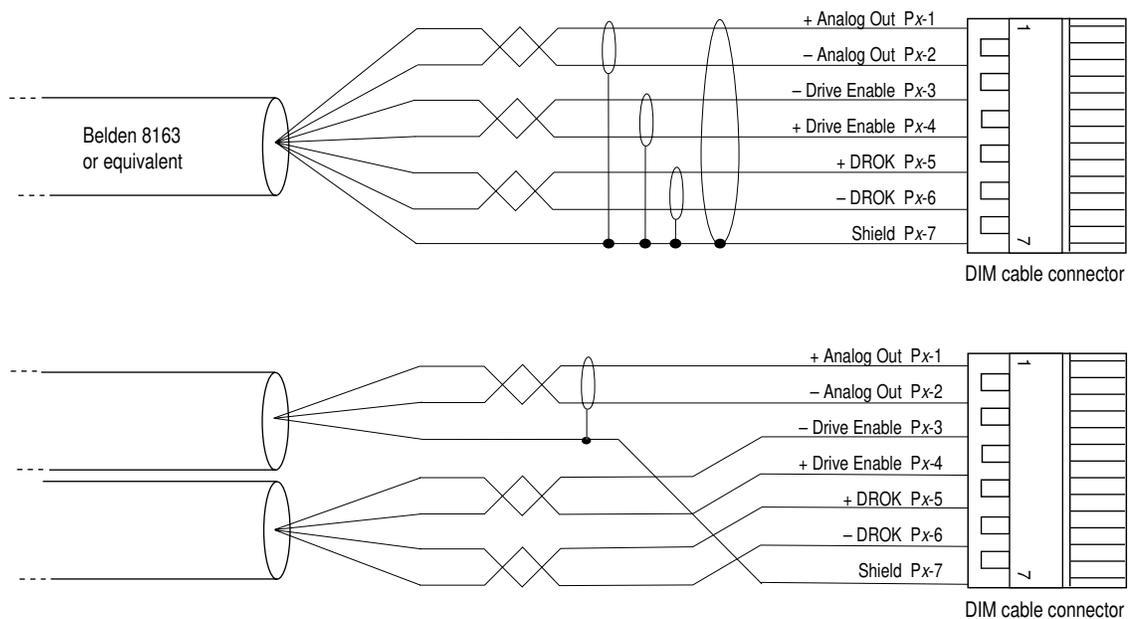
To wire the cable flying leads to the DIM cable connector:
