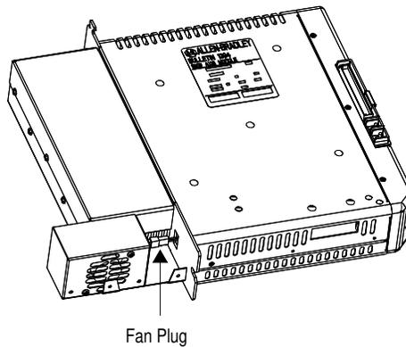
8. Slide the fan housing back into place.
