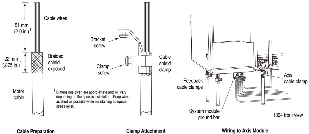
2. Prepare one end of the motor cable for attachment to the cable shield clamp by removing the outer insulation and braided shield from the motor cable. Ensure approximately 51 mm (2.0 in.) of the insulated cable wires are exposed (refer to Figure 3.14).
