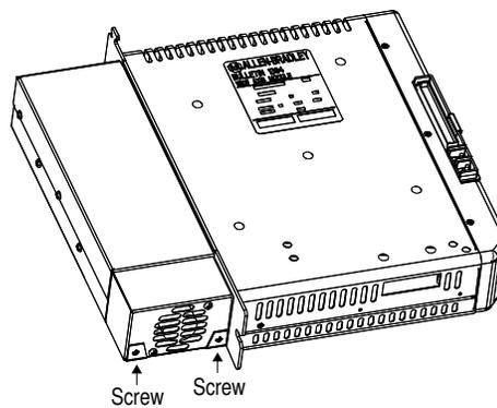
5. Gently slide the fan housing out a short distance until you see the fan plug.
