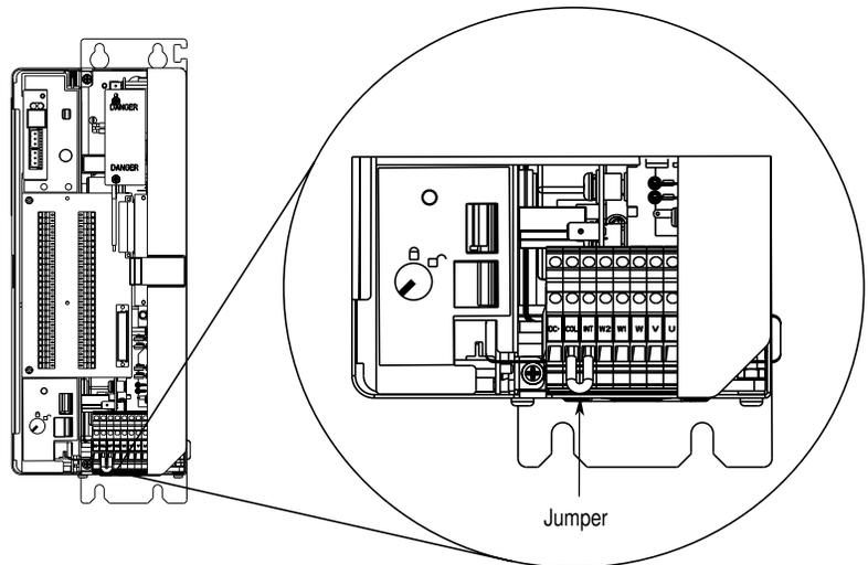
3. Install the jumper block in the P1 position, which is located directly behind the Status LED, as shown in the figure below.
