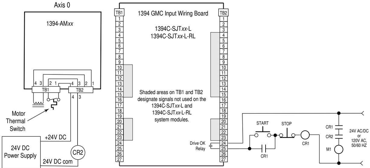
Note: 120V AC (50 or 60 Hz) power may be used in place of a 24V DC power supply for the motor thermal switch circuit.
