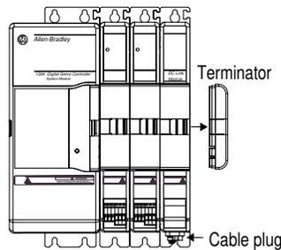
3. Remove either the power plug from the stand-alone 1394-DCLM (shown above) or remove the cable linking two systems together, as shown below.
