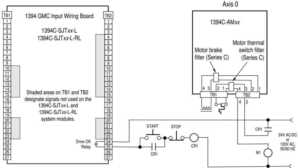
The example below shows a 1394 (Series C) axis module wired for thermal fault monitoring. The fault can be used to monitor or disable the axis.
