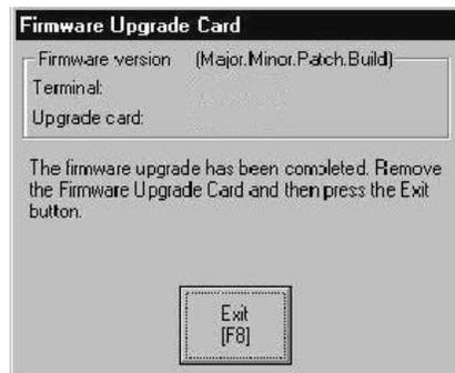
7. Communication settings are cleared when the terminal is upgraded. If Ethernet communications is used, reconfigure the Ethernet communication settings using the values recorded when preparing the terminal.
