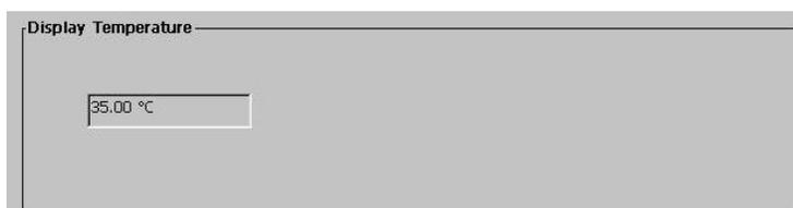
The terminals have a CCFL (Cold-Cathode Fluorescent Lamp) backlight. This backlight requires temperature control when the internal temperature of the product is below 10 °C or above 60 °C. For proper backlight operation, the terminal monitors low and high temperature conditions.
